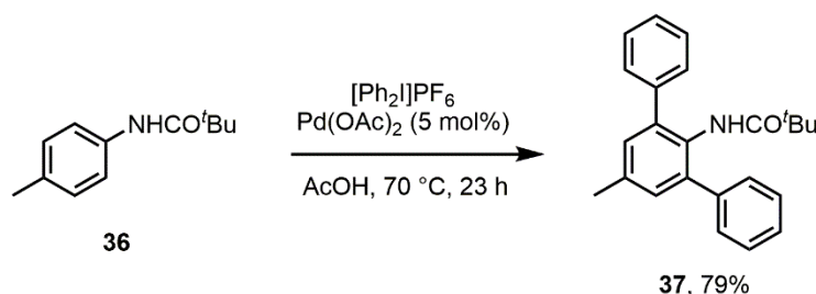
Scheme 19 Anilide-directed ortho -arylation using diaryliodonium salts.
