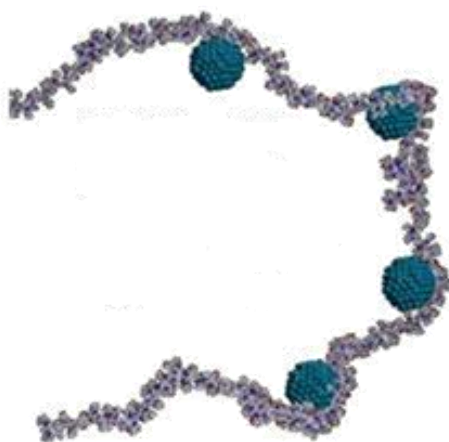
Figure 20 Cartoon schematic of PdNP encapsulation in PVP–Pd 13 .
