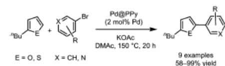
Scheme 27 Direct C2-arylation of furans and thiophenes with bromoarenes using a Pd-polypyrrole nanocatalyst (Hierso et al., 2011). 108
