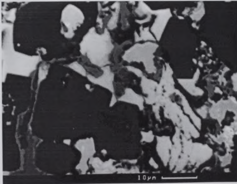
Figure 6.62 BSE image of metallic iron (light) and CaS (dark) formation from the reduction of chalcopyrite with 1 wt.% Ag at 1150°C for 180 minutes.
