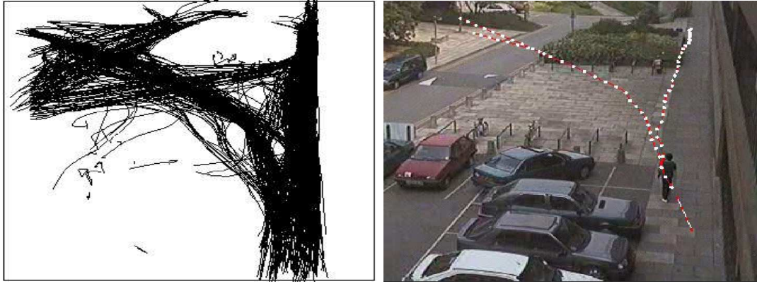
Figure 2.11: From observation of many trajectories the system is able to predict the path of a pedestrian.
