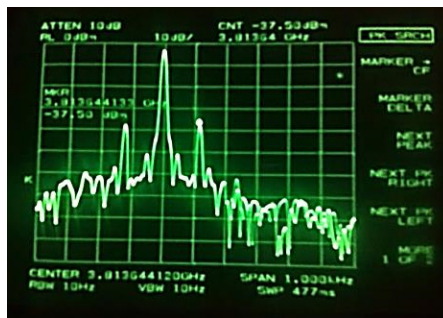
Figure 3.41: Sidebands seen on a spectrum analyser due to vibrations at 120Hz for a_i=0.14g .
