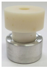
Figure 3.15: The dielectric puck was mounted on a short alumina spacer and then bonded to the aluminum base using two-part epoxy.
