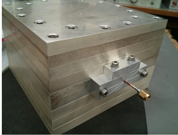
Figure 5.2: Aperiodic 6 plate Bragg Resonator with the clamping mechanism
