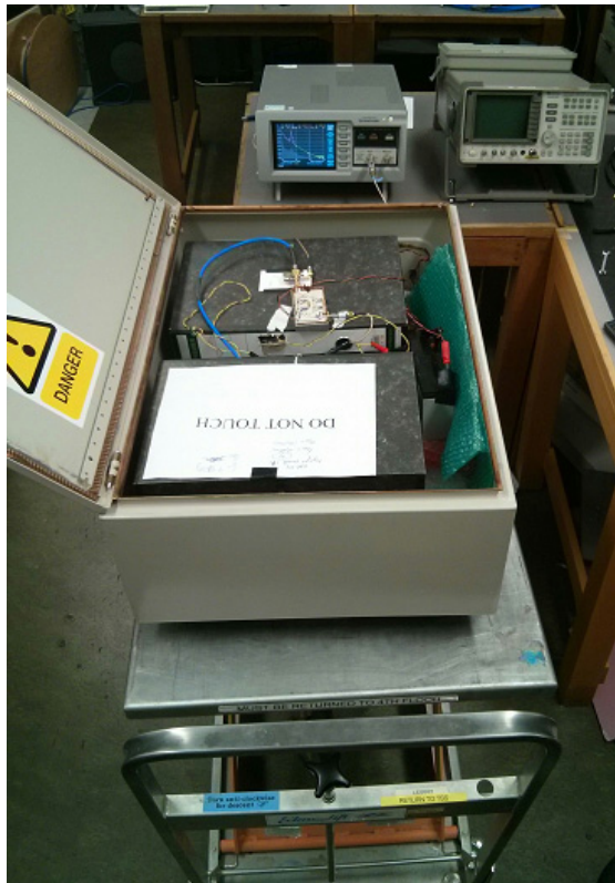
Figure 5.29: 10GHz battery operated oscillators screened in a metal box and resting on a set of tubes in order to dampen any mechanical vibrations.
