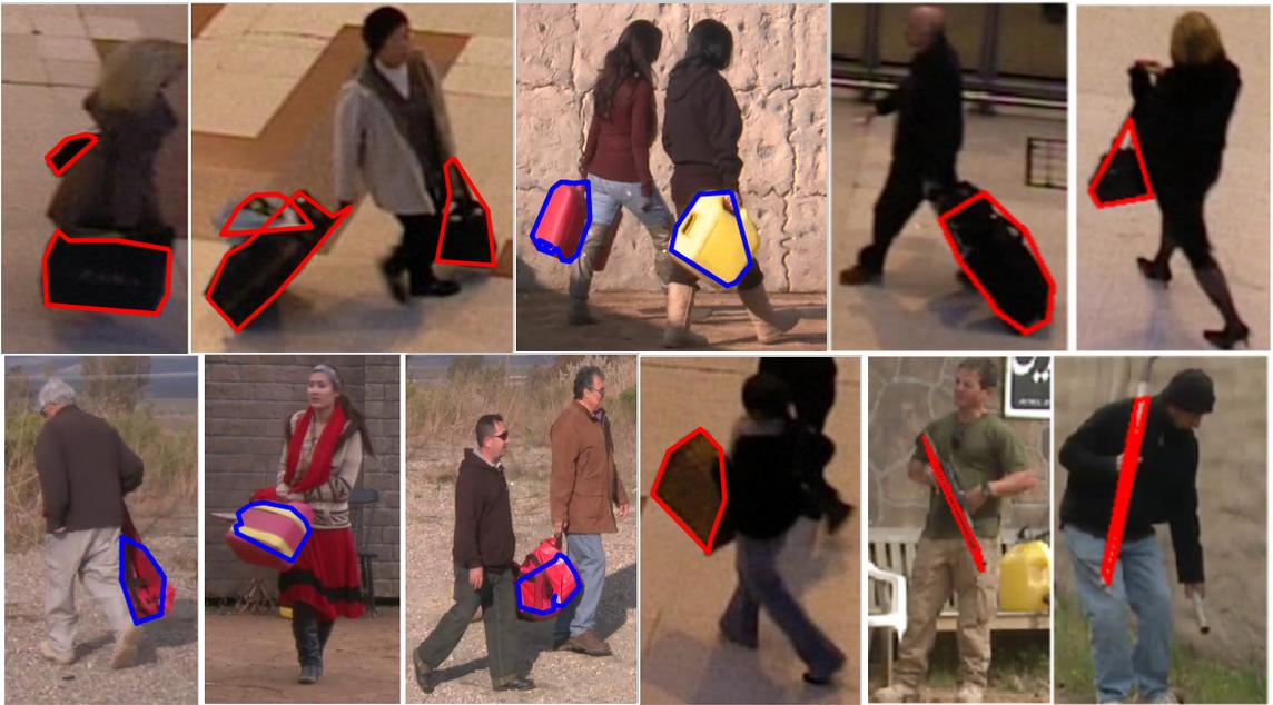
Figure 3.13: Example output boundaries of our carried object detector across different datasets. Each boundary is displayed as a connected chain in red or blue for a better contrast with respect to the object colour or background.
