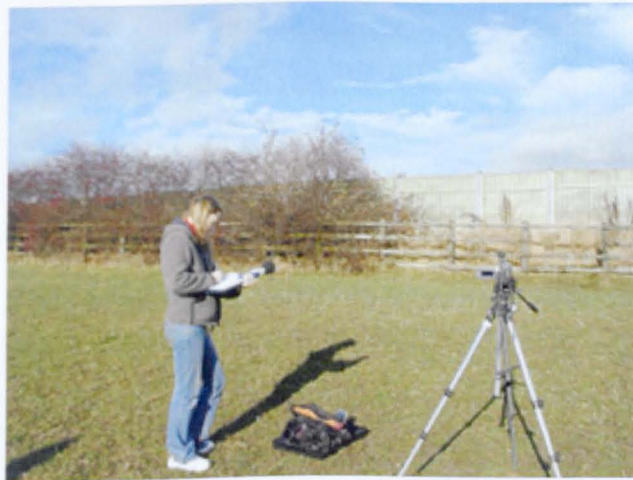
Figure 8.1. Recording visual and audio sequence and noise levels behind the reflective concrete barrier (Nr Junction 33 Northbound M1).
