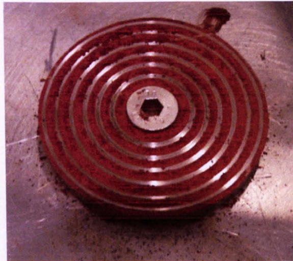
Figure 79 image showing wear scars on 100% oxide disc specimen
