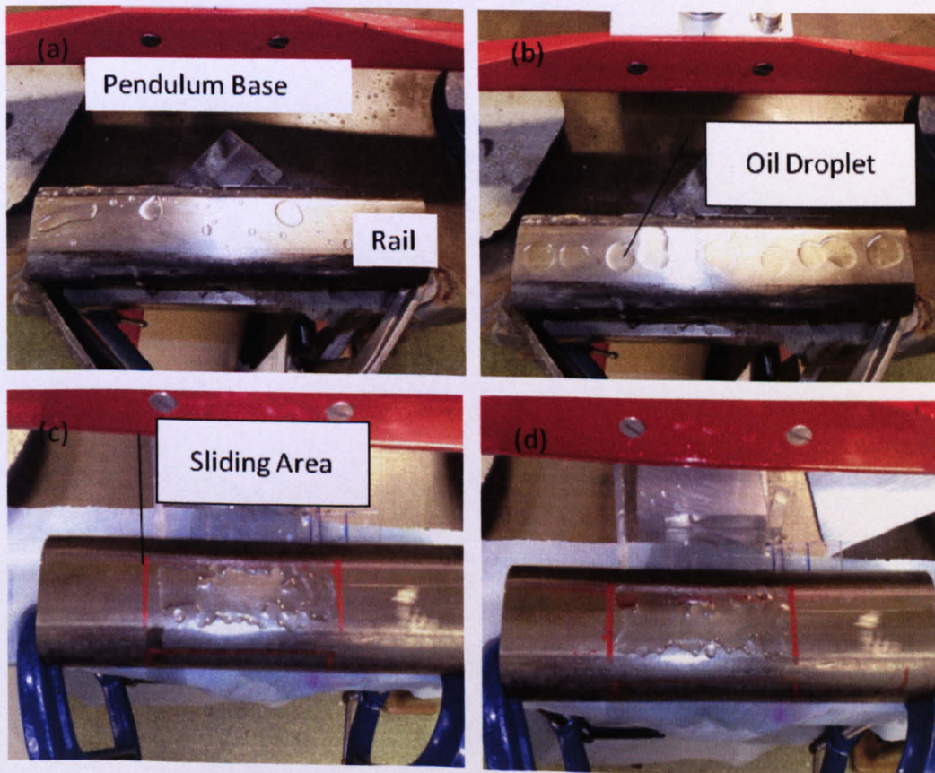
Figure 24 a) water spread along rail, b) oil dispersed along rail, c) water dispersed within marked contact area, d) oil dispersed within contact
