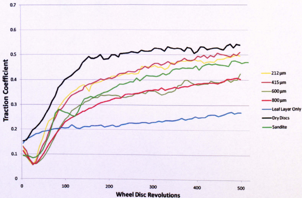
Figure 51 traction curves for first series of tests (fixed volume of gel)
