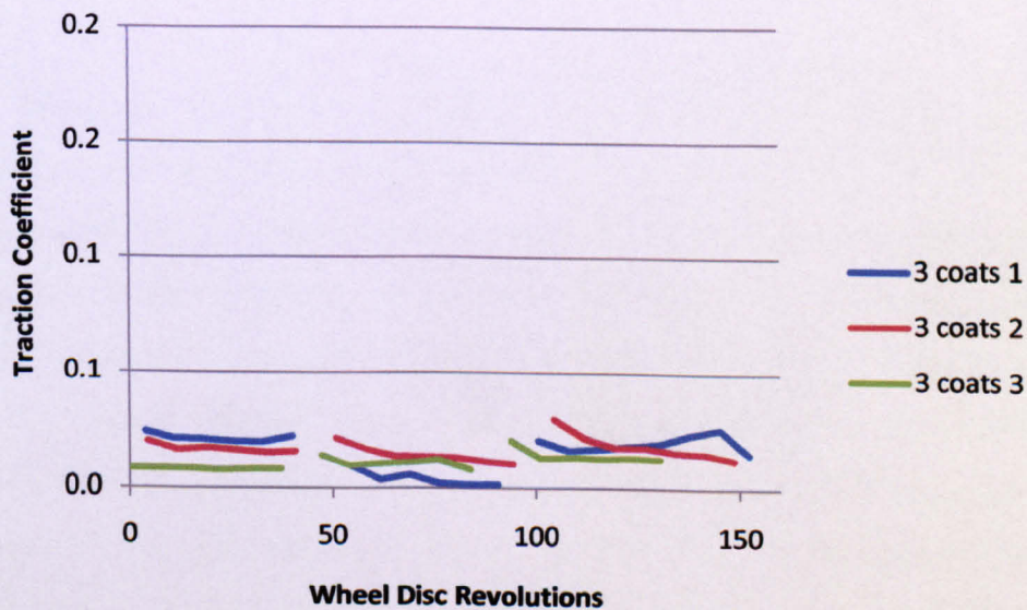
Figure 50 traction curves recorded during generation of leaf layer
