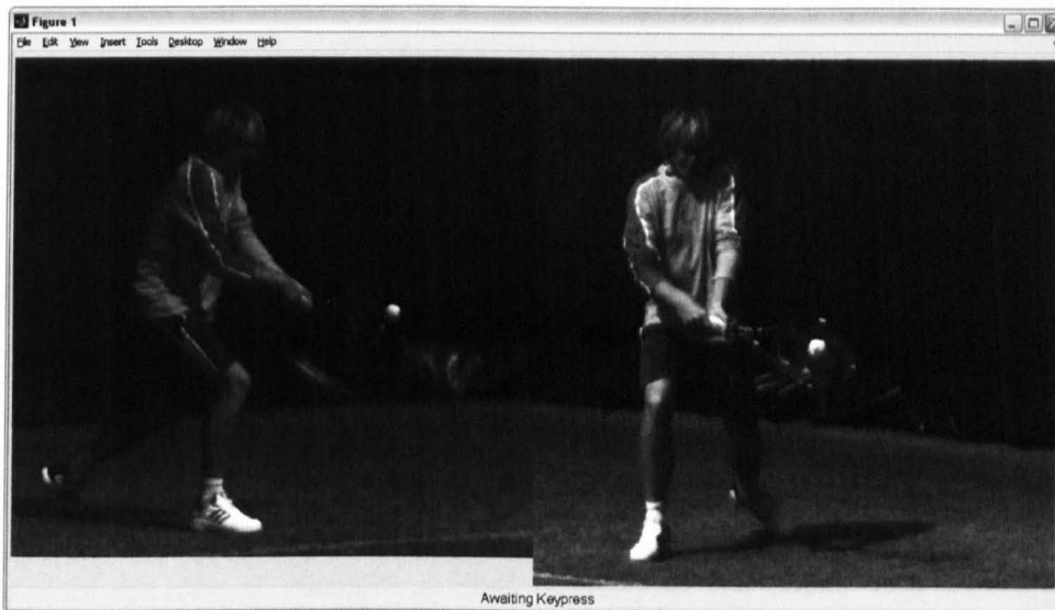
Figure 4.18. The 2D point extraction program. After the images from each camera are loaded into it, they are displayed adjacently as shown here.
