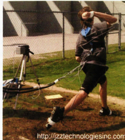
Figure 2.12. The accelerometer based system by JZZ technologies. A physical connection of the athlete to the recording system prohibits any large movements by the athlete.
