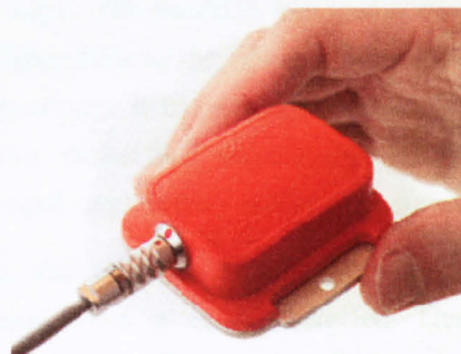
Figure 2.13. One of the accelerator/gyroscope units used in the moven full body motion capture system developed by Xsens 2007.
