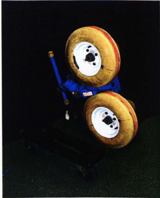
Figure 3.5 Picture of the pitching machine mounted on a custom built stand used for projecting the tennis balls up to 100mph
