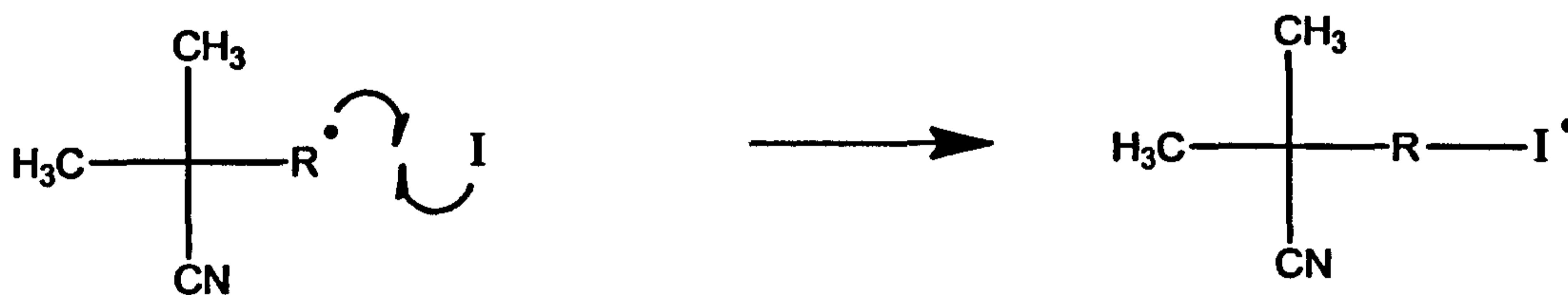
Figure 16: A final termination possibility would be reaction with an inhibitor species, shown as I, which forms a much more stable radical species in effect stopping further polymerisation possible inhibitors could be oxygen molecules or large aromatic species both of which will form much less reaction radical species at the chain end.
