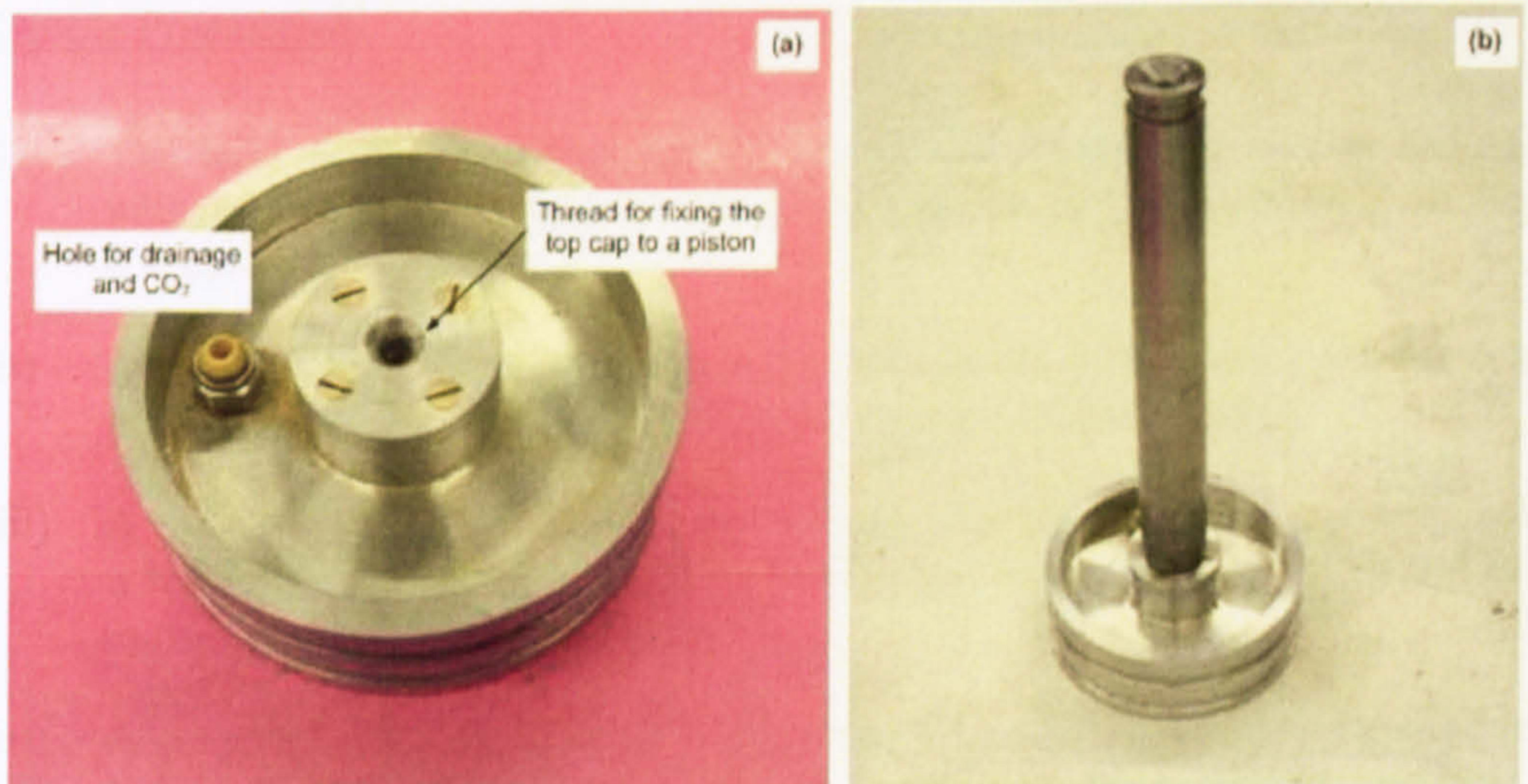
Figure 4. 3 Top cap and piston for undrained monotonic triaxial extension test
