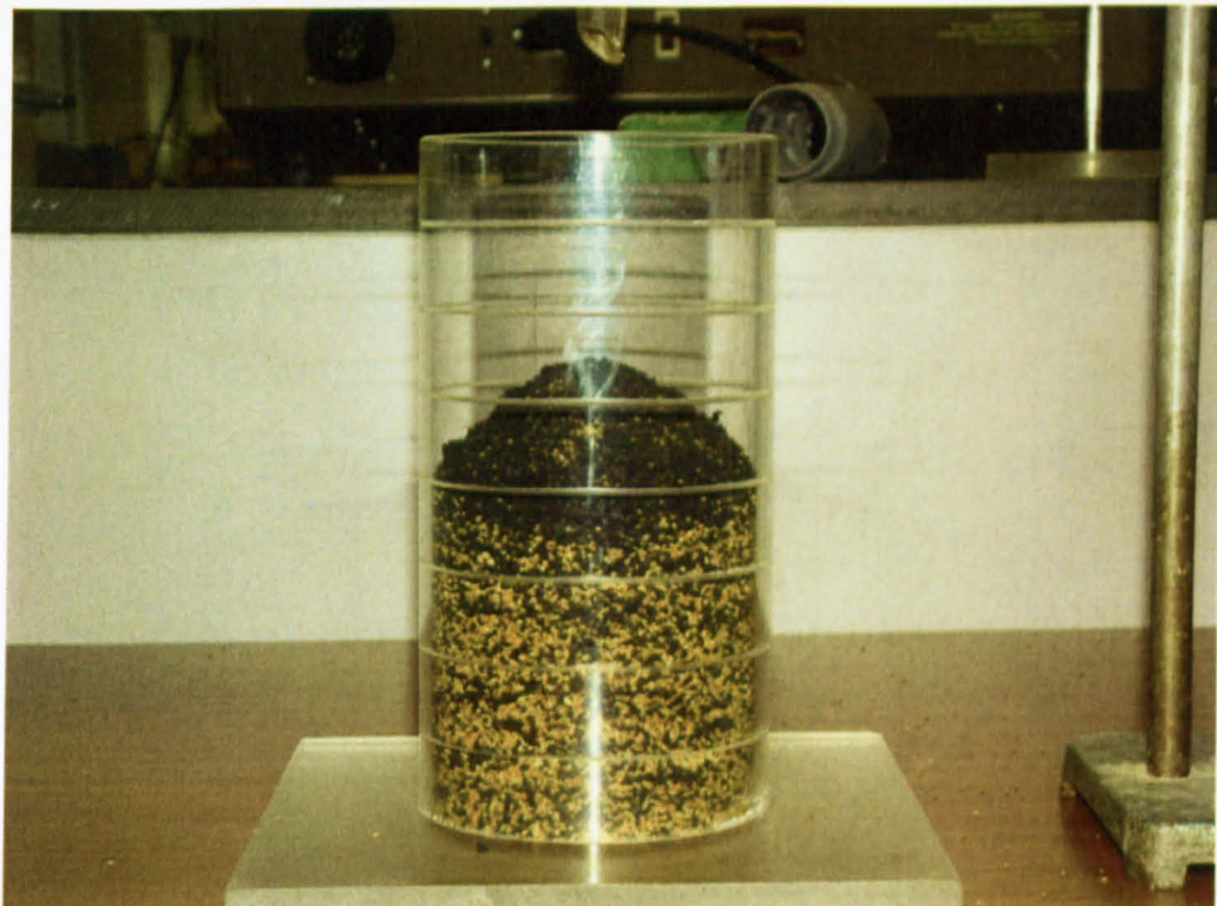
Figure 3. 7 Segregation of sand mixed with tyre chips
