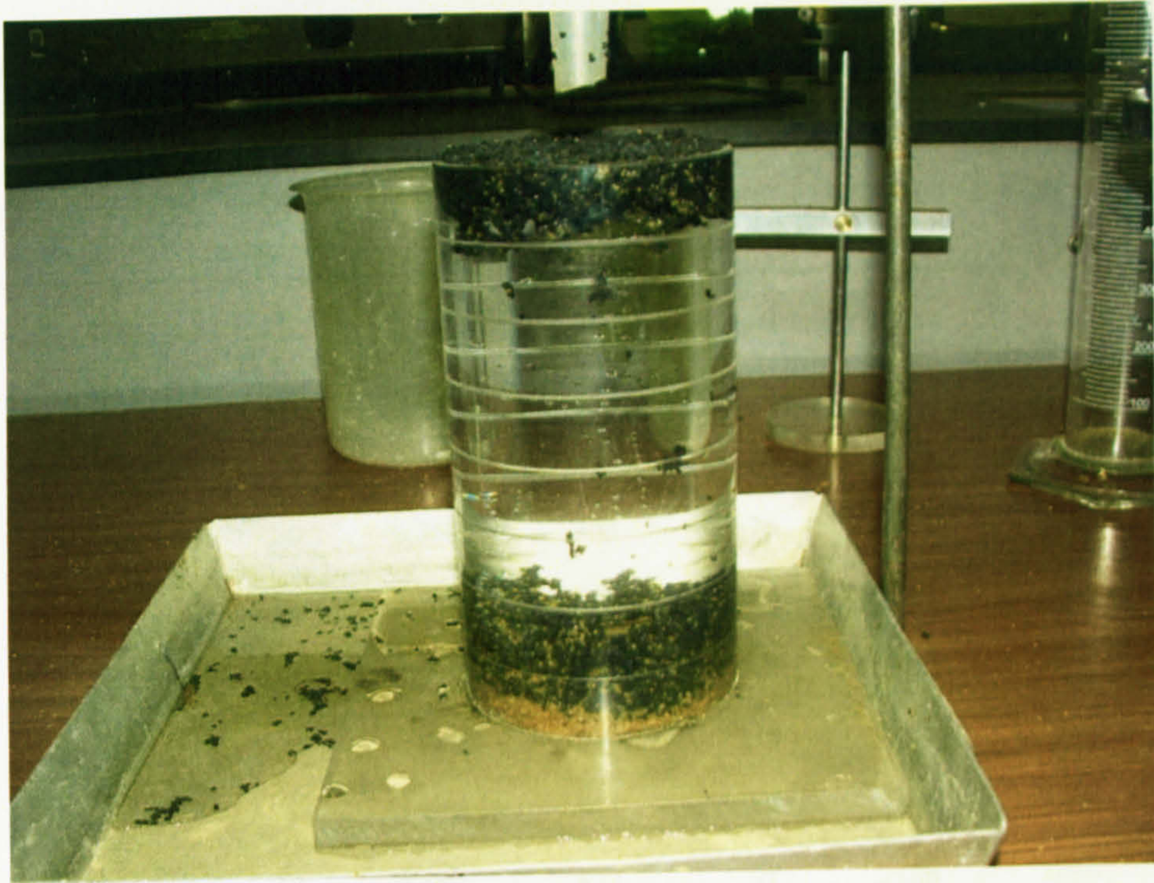
Figure 3. 8 Tyre chips floating due to air trapped around their edges
