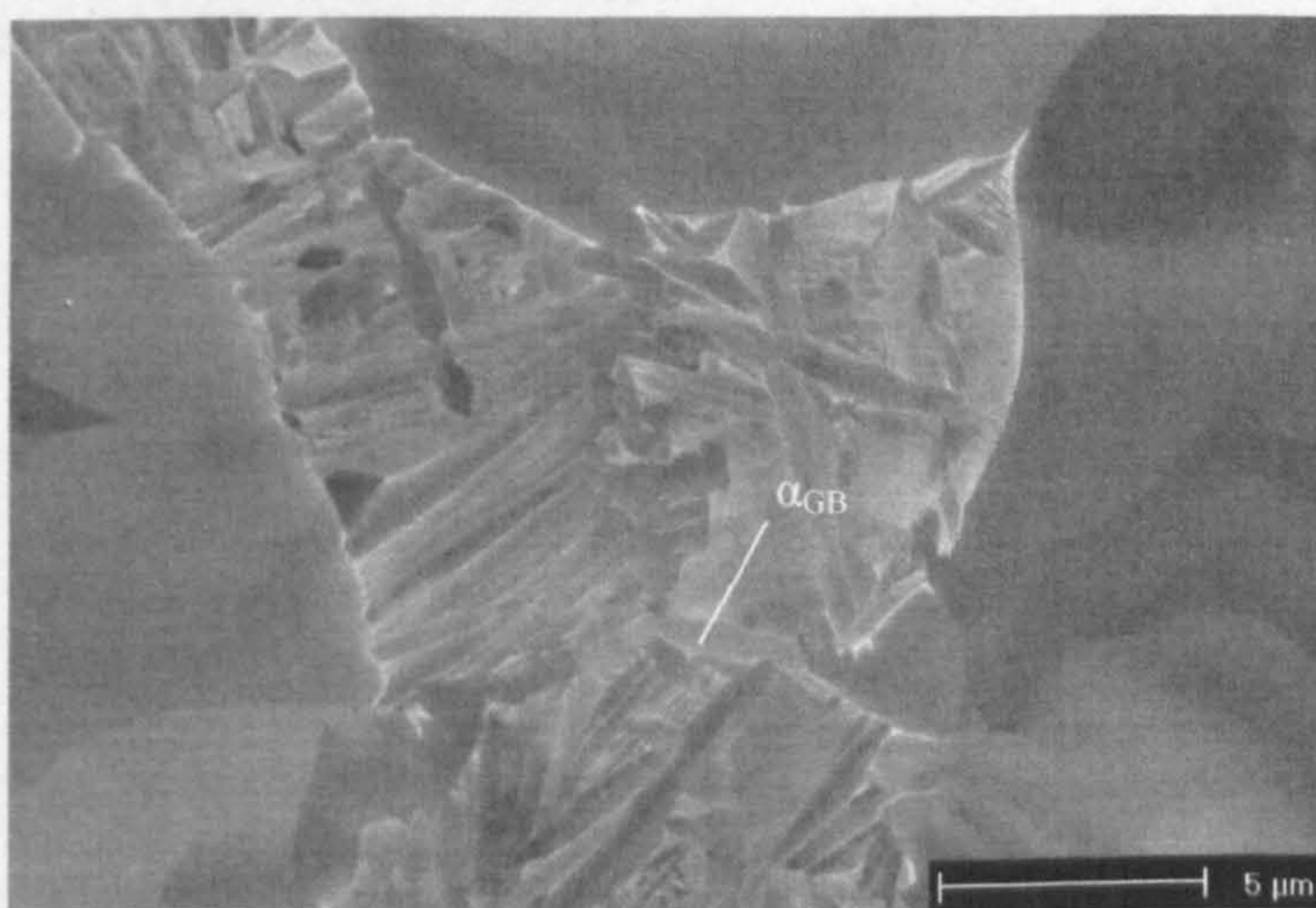
Fig. 7.34 BSE image 7mm from quenched end, CR_{900} = 30^\circ\text{C s}^{-1} .
