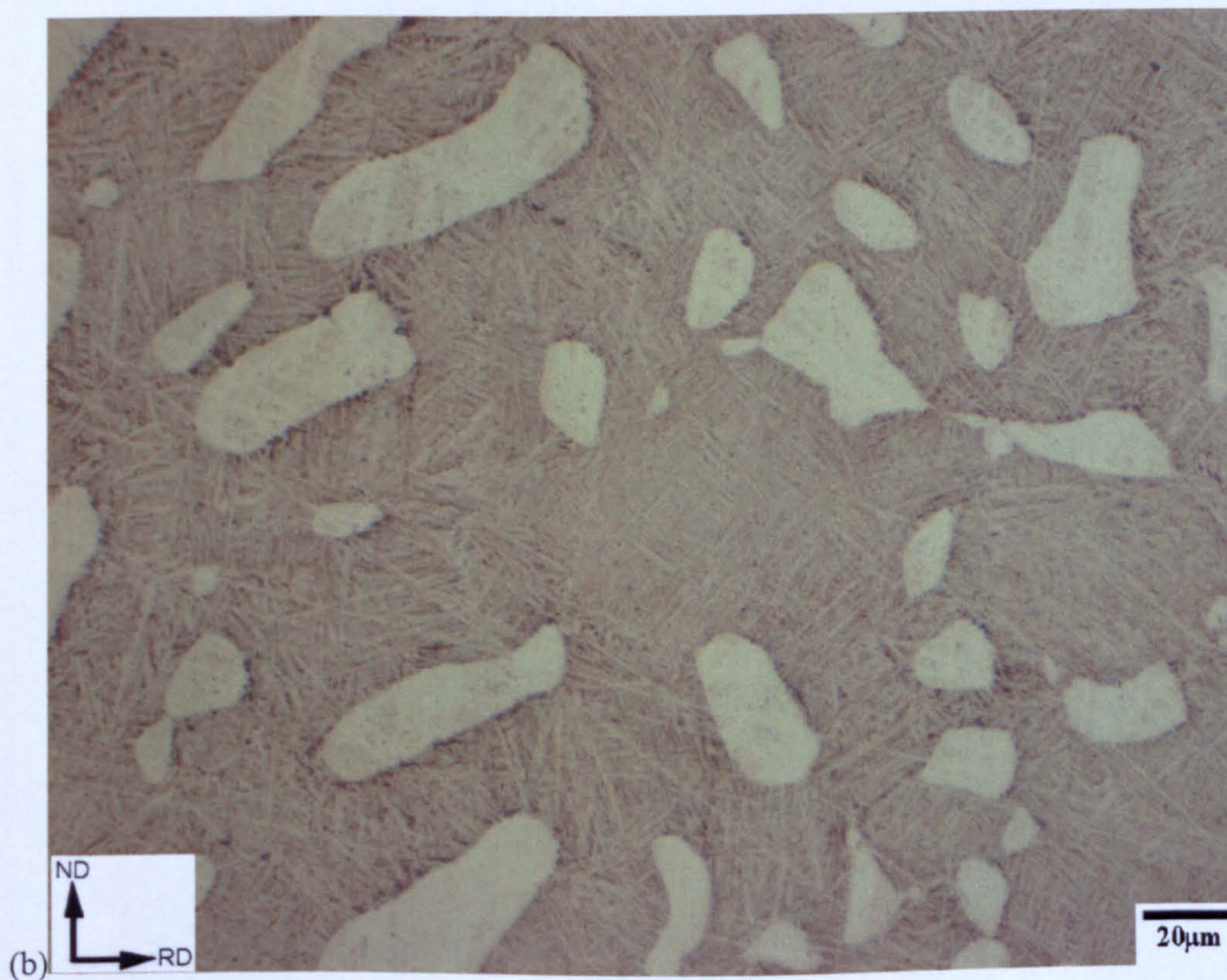
Fig. 8.26 Optical micrographs from specimen F, which was deformed at a true strain rate of 0.019\text{s}^{-1} , to an equivalent true strain of 0.67.
