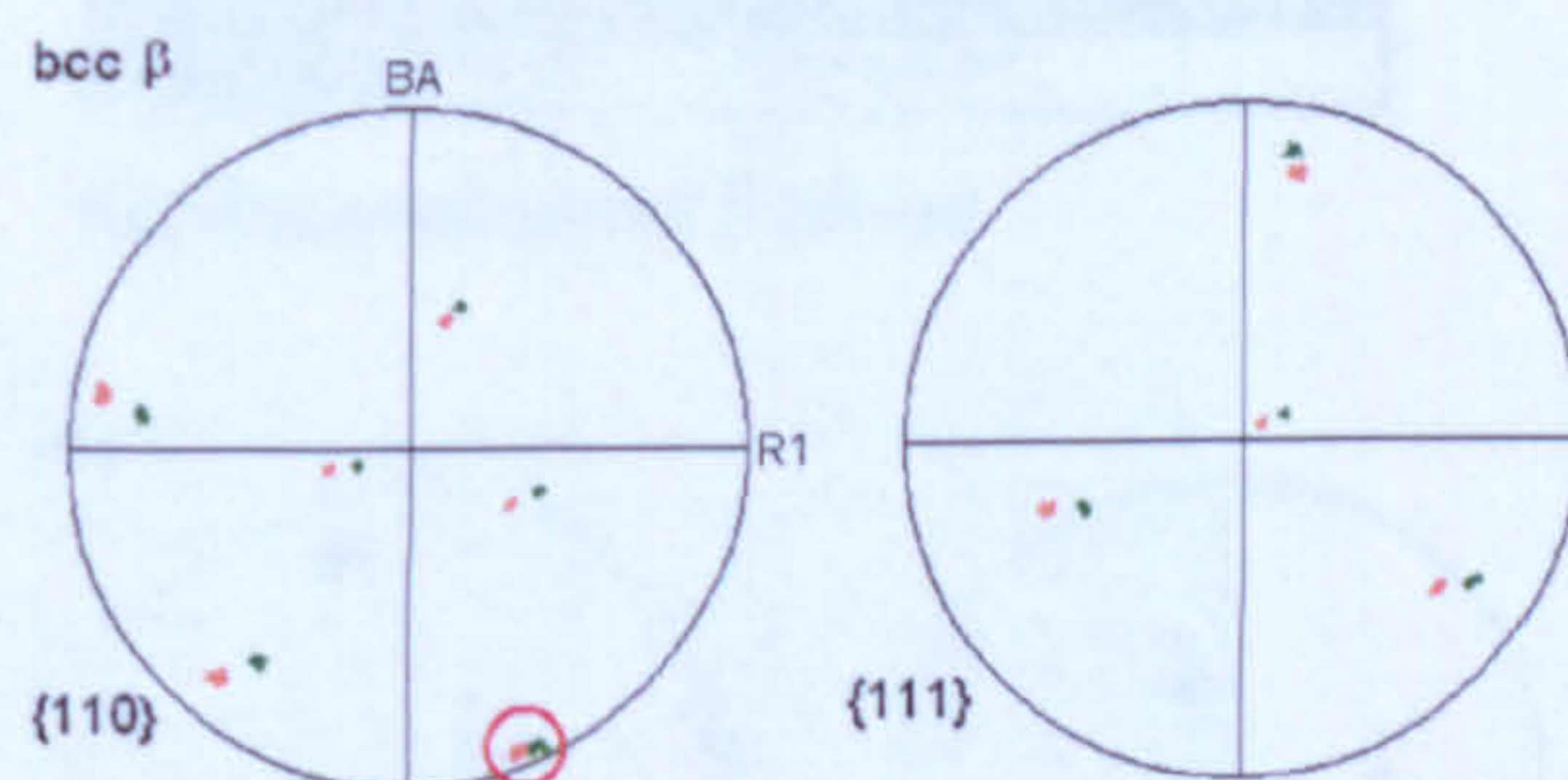
(f) Cubic pole figures for adjacent \beta grains \beta_1 and \beta_2 .
