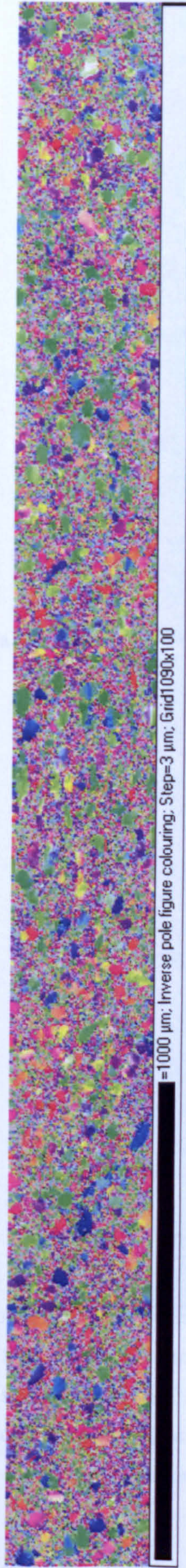
Fig. 8.30 Low resolution EBSD analysis from specimen C, deformed at a true strain rate of 1.8\text{s}^{-1} to an equivalent true strain of 1.23 (71% indexed).
