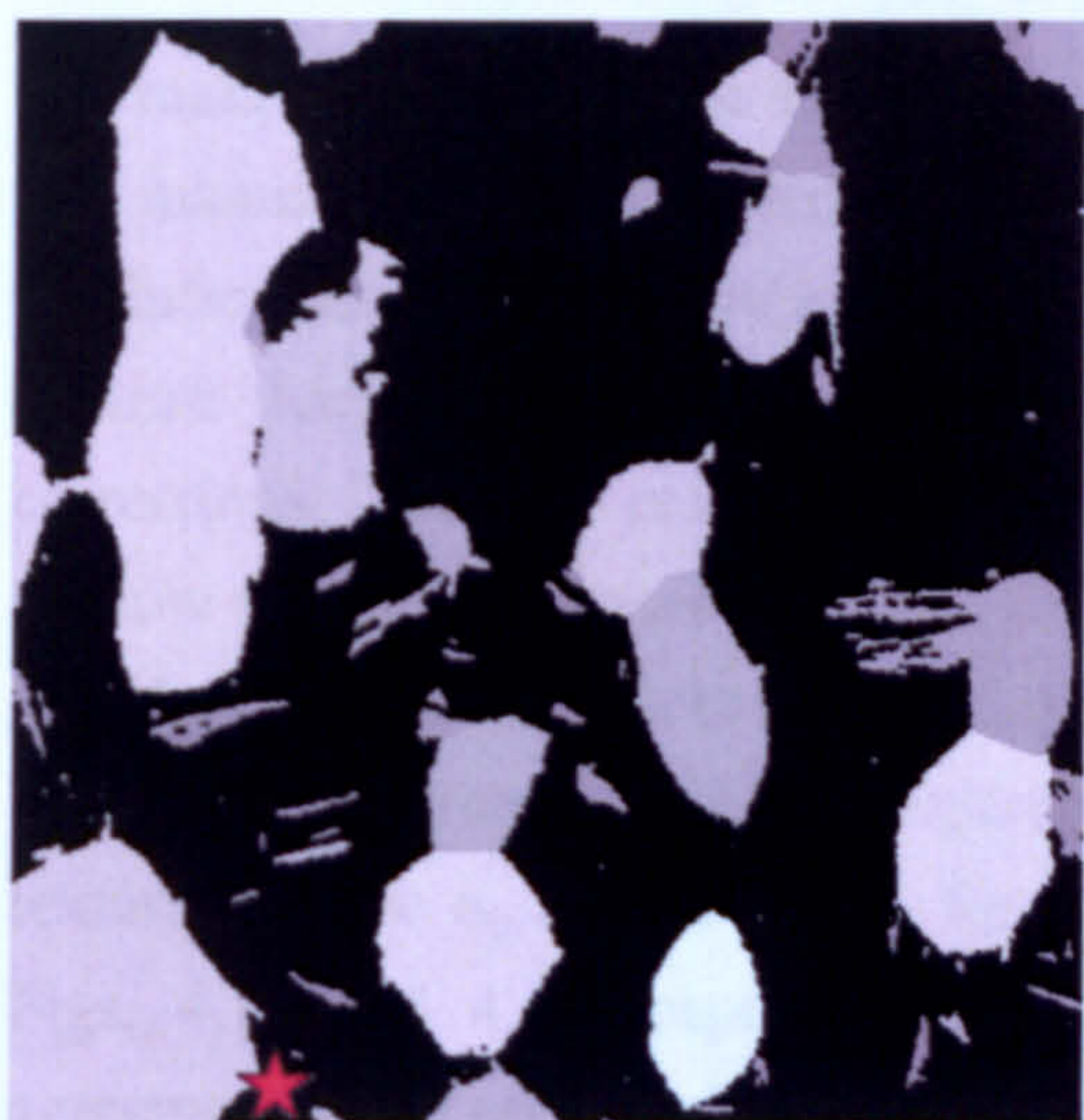
(e) Step 1: removal of grains below a threshold gray level (180). Removed \alpha_p grain indicated.
