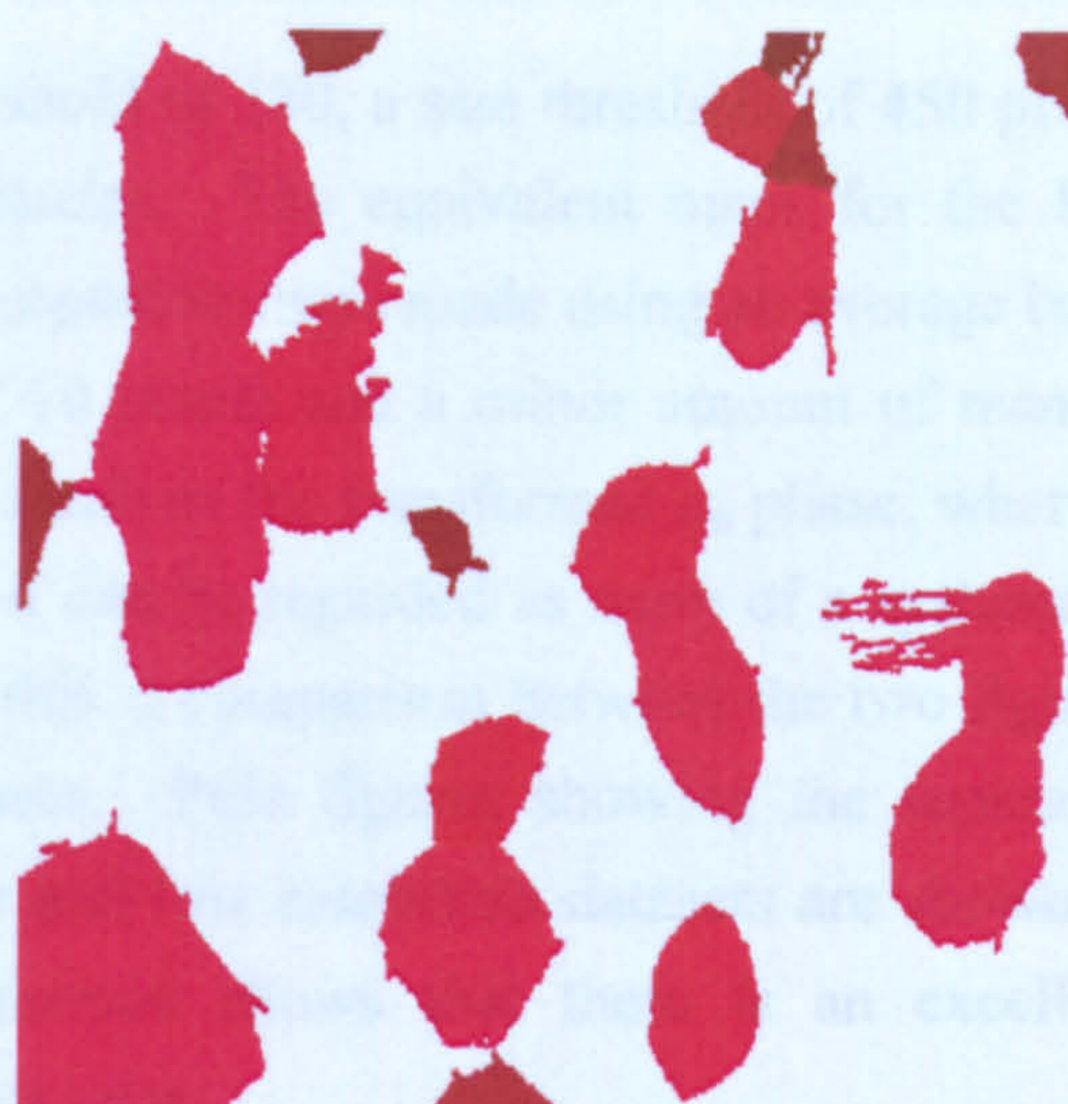
(f) Step 2: removal of grains below a threshold size level (450 pixels).
