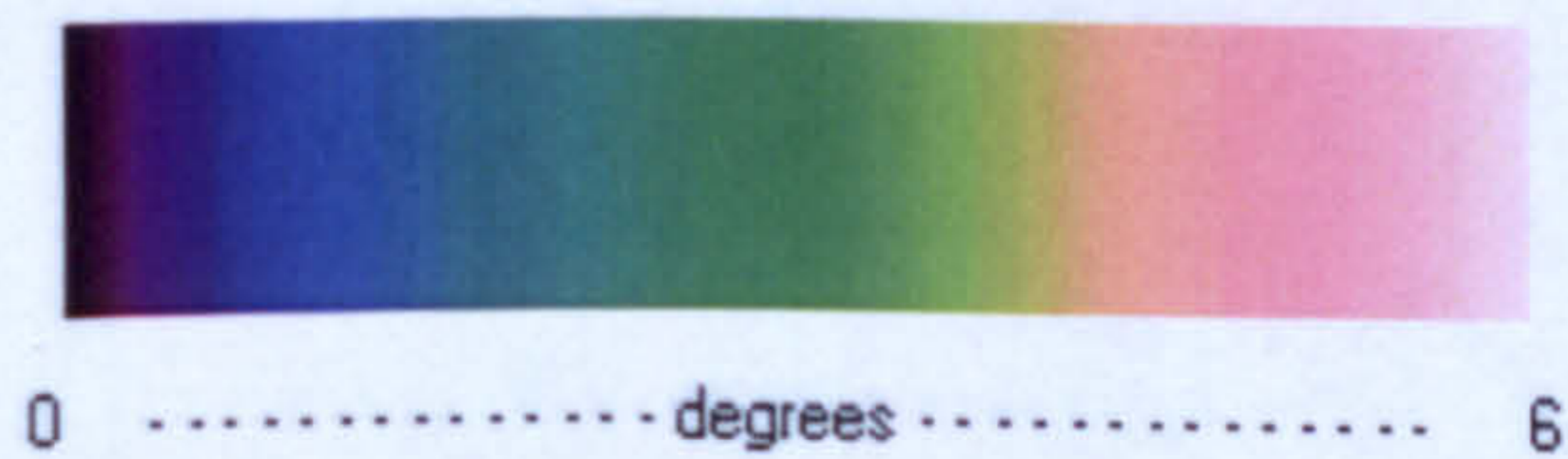
(c) Misorientations > 3^\circ are coloured according to their deviation from the Burgers relation. Deviations > 6^\circ are coloured white.
