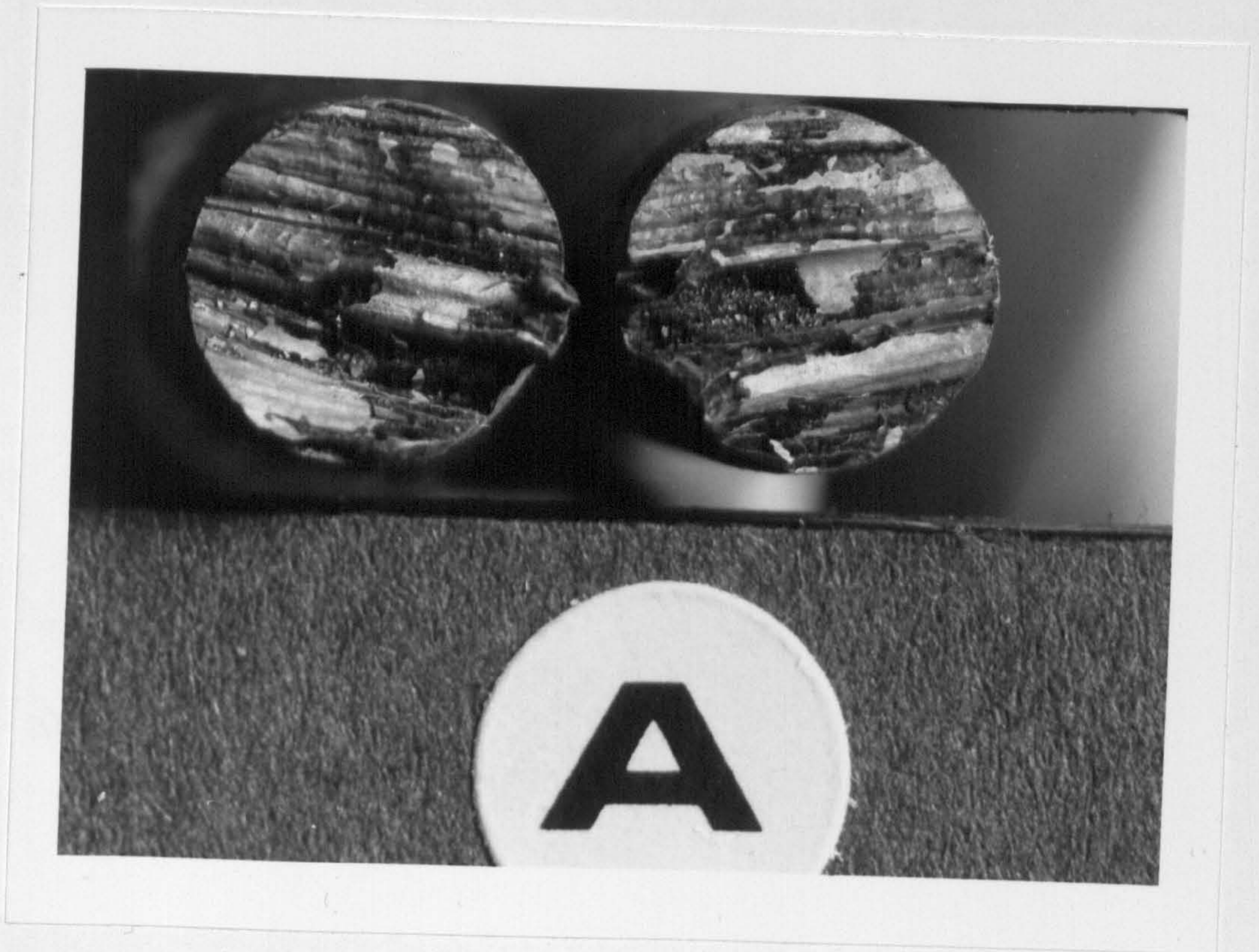
Figure 3.25: Fracture surfaces for specimen (A), Fig.3.24, tested at 500°C.
