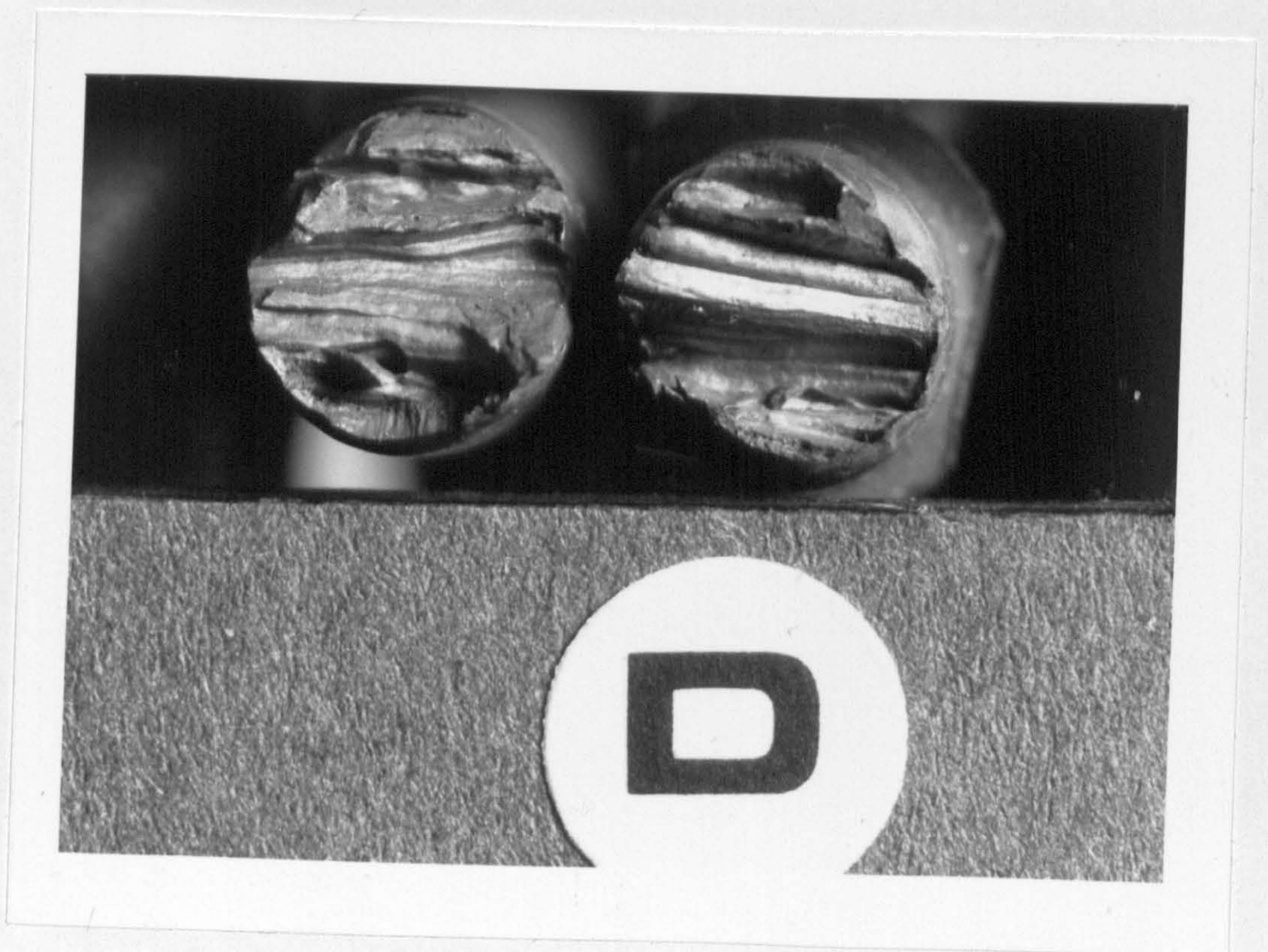
Figure 3.26: Fracture surfaces for specimen (D), Fig.3.24, tested at 250°C.
