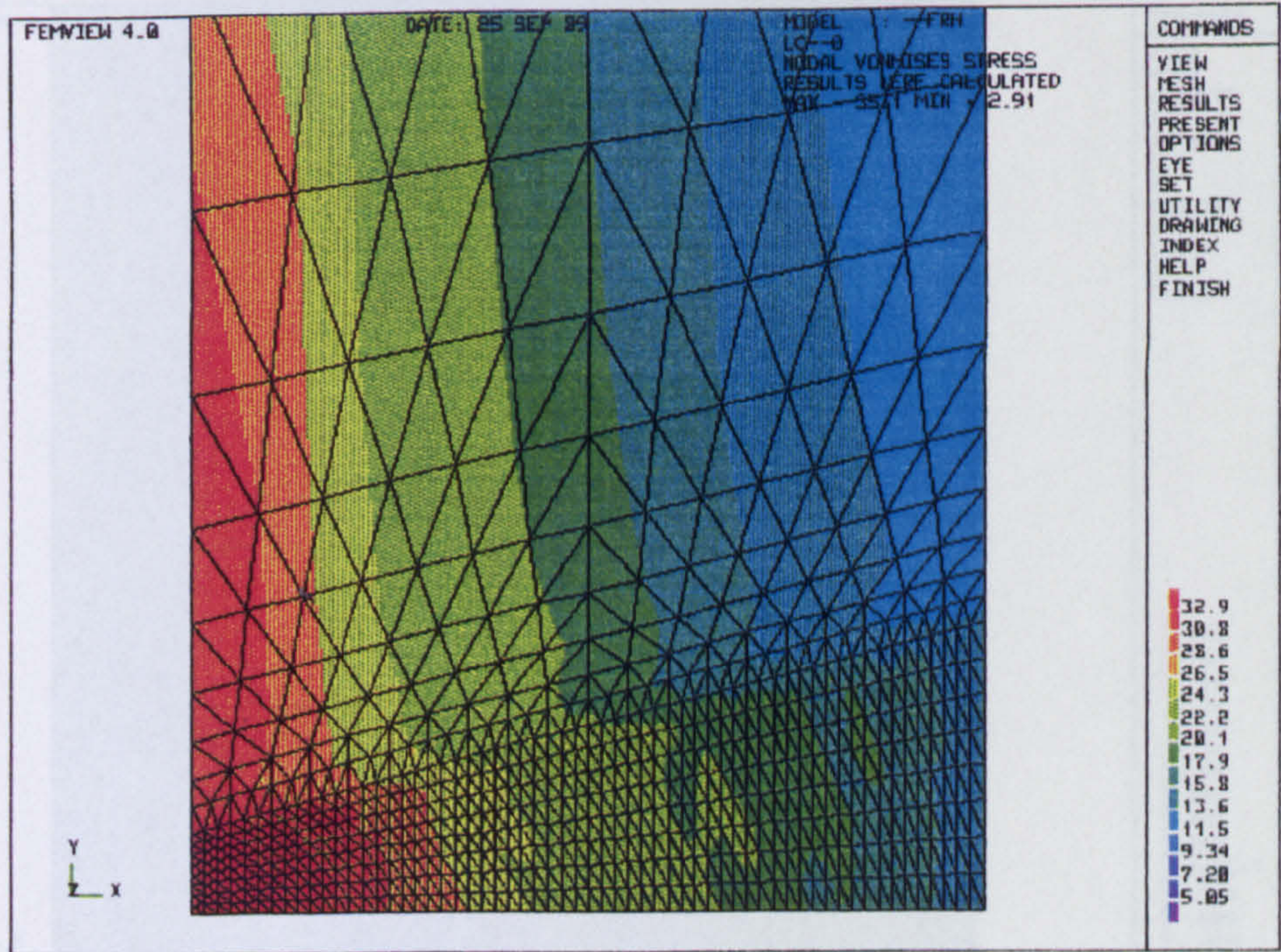
Figure 8.98: Distribution of the normalised Von Mises (effective) creep strain ( V_{ef} = V_{ef}/\sigma_o ) for weld model (WM3) at a life fraction of ( t/t_f = 99.9\% ).
