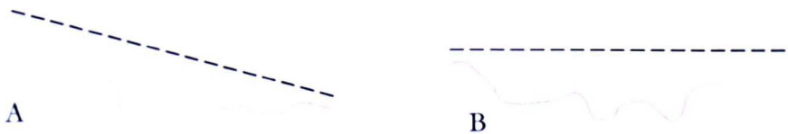
Figure 2.47 Diagram showing two identical traces (A) without Least Square levelling and (B) including Least Square levelling
