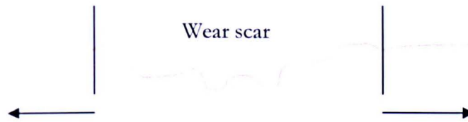
Figure 2.46 Diagram showing form fit exclusion. Data behind the black lines (indicated by the arrows) are excluded from the measurements
