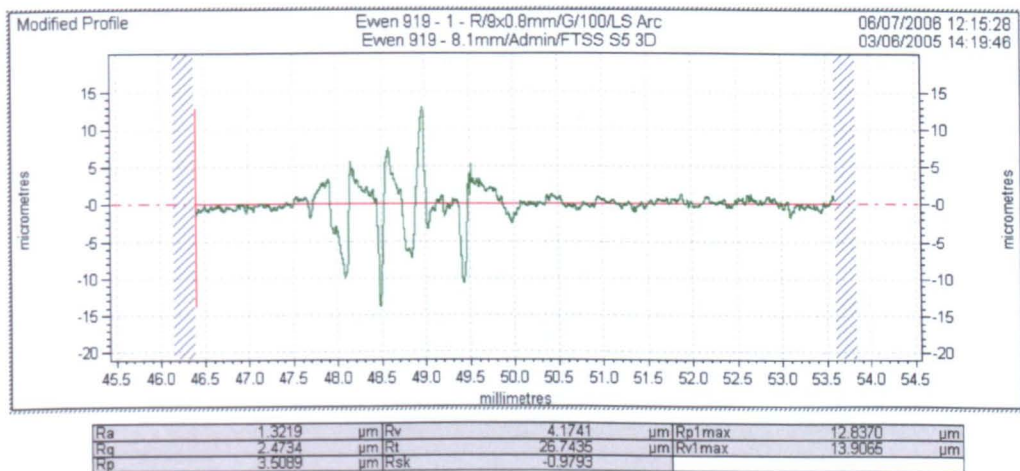
Figure 5-2: Example of a Surface Profilometry trace for an initial pin at 0 minutes
