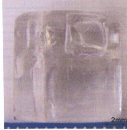
Figure 3-26: Internal fractures to hydrogel 1D following non-confined compressive test at 1.5 MPa Contact Pressure
