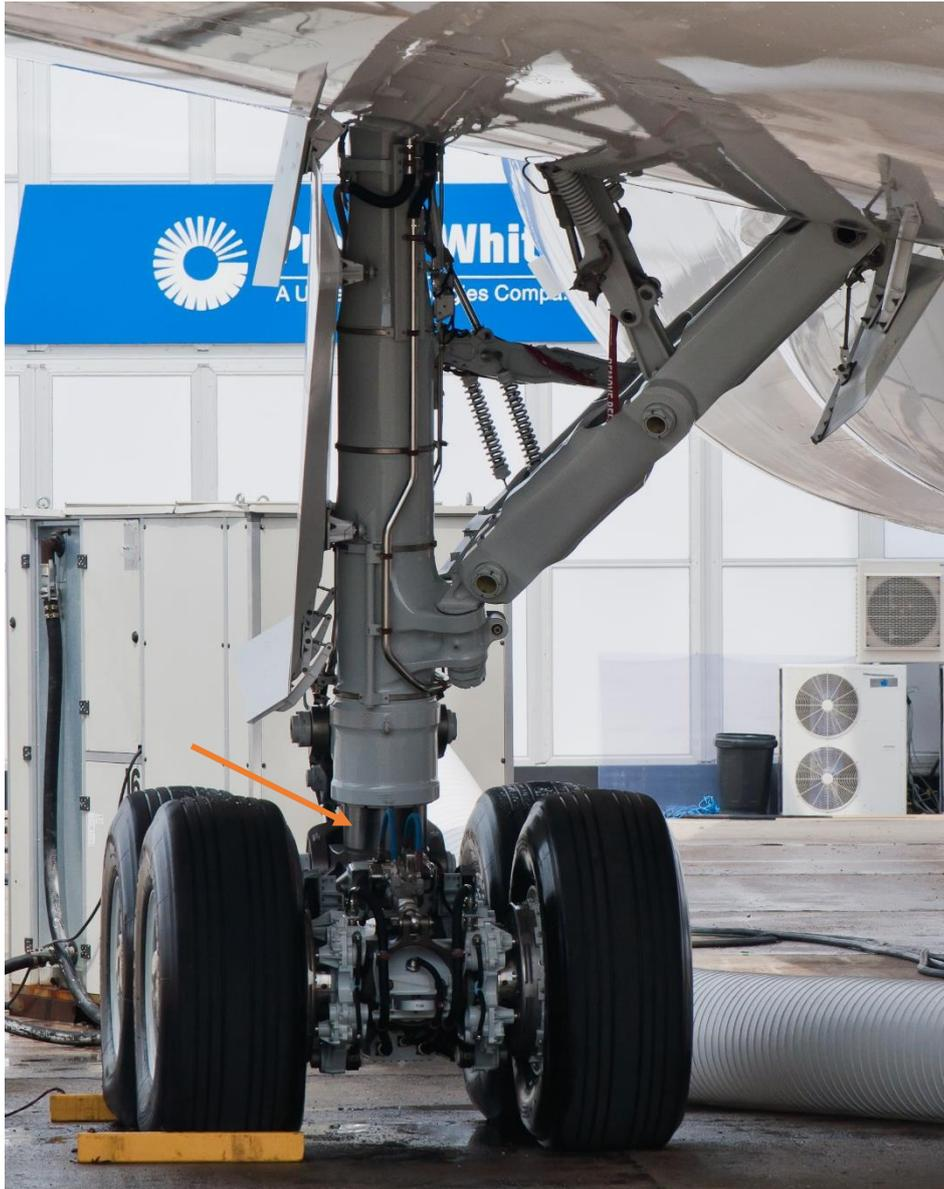
Figure 4.1: Right-hand main landing gear of a Boeing 787. Arrow indicates the inner cylinder. Photograph by Julian Herzog, taken at the Paris airshow, 19<sup>th</sup> June 2013 and shared under a creative commons license (4.0). Image has been cropped to fit.
