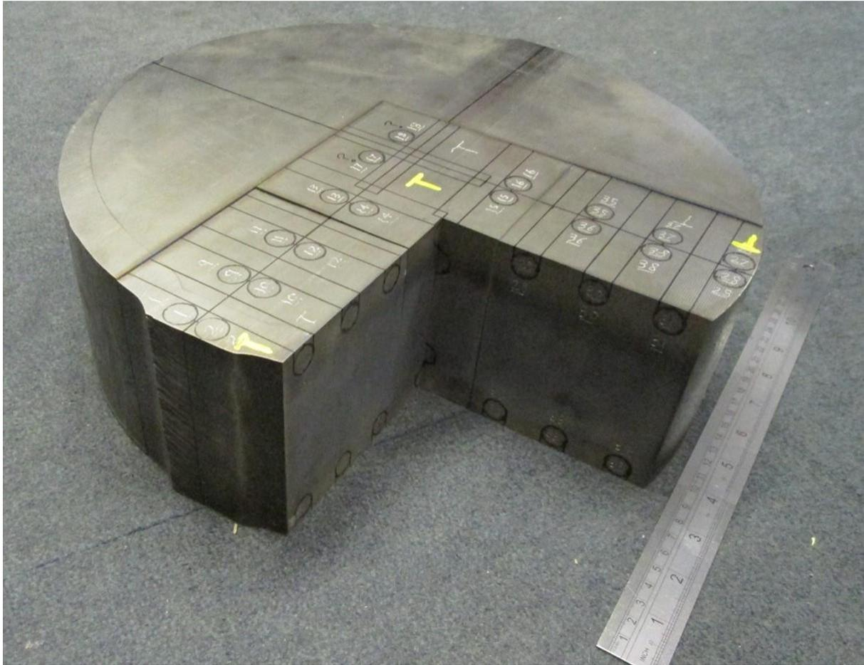
Figure A. 1: Forging 2, with specimen locations marked for removal via EDM.
