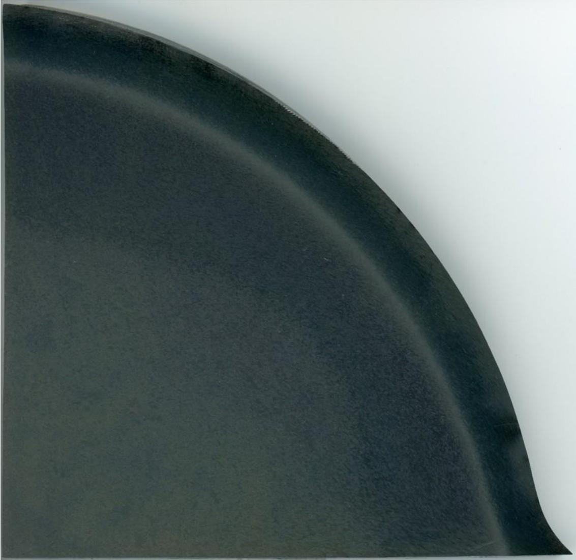
Figure A. 4: Unedited scan of quarter cross-section macro-etch
