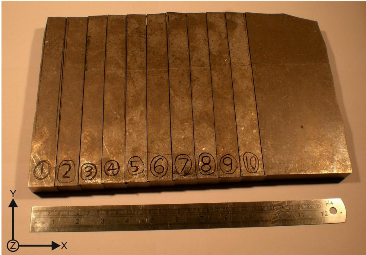
Figure 5.1: Ti-10-2-3 as-received material after sectioning (305 mm ruler)
