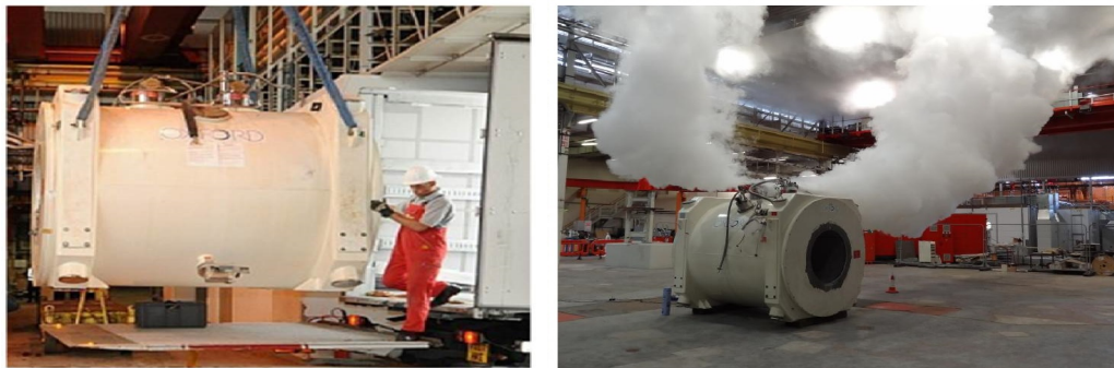
FIGURE 1.12: (Left) The world first hospital MRI scanner was moved from the University of Nottingham to Daresbury Laboratory for preliminary tests. (Right) MRI scanner was being cooled with liquid nitrogen in Daresbury Laboratory. A magnetic field measurement could not be successfully carried out because of quenching, followed by the termination of liquid nitrogen a few minutes later.
