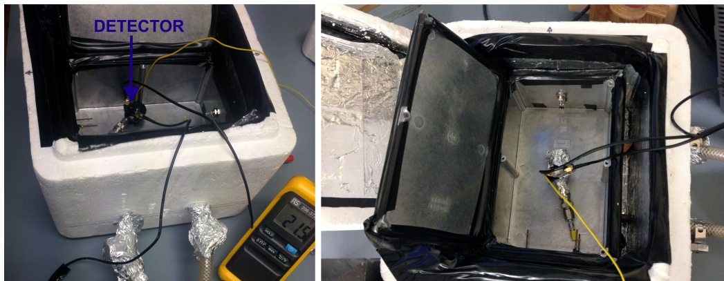
FIGURE 3.7: Detector system set-up inside the thermally-isolated temperature controlled chamber. (a) A Fluke digital thermometer probe was attached to the sensor board by a black tape, and it was then placed inside the chamber. (b) A thermally isolated lid was used to cover the chamber after the experimental set-up was completed.
