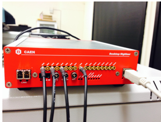
FIGURE 4.5: Picture of a DT5742 desktop waveform digitiser with 16 channels, a trigger, and other connections. A CAEN Waveform digitiser was used to obtain accurate and very fast time measurement (which can achieve few picoseconds time resolution).
