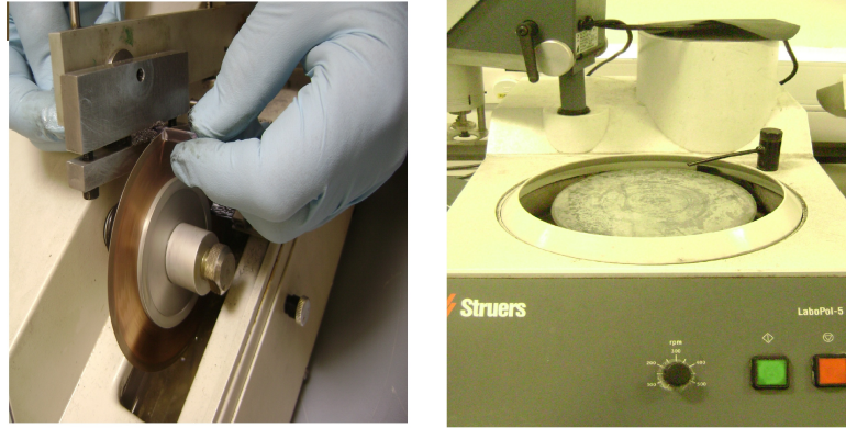
FIGURE 2.18: A diamond wheel saw cutter was used for cutting LYSO and BGO sticks without damaging the crystals (left). A lapping machine was employed to make the cutting face of crystals smooth (right).
