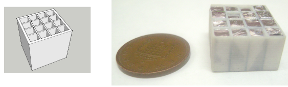
FIGURE 2.19: An example of an array grid was drawn in Google SketchUp 3D modelling software program with a size similar to the crystals. The array was obtained from a 3D printer. The main material of the grid was plastic. 4.5 \times 3 \times 10 \text{ mm}^3 LYSO crystals were placed inside the grid after being covered with several layers of PTFE (thread seal tape 0.075 mm thickness Teflon based reflector [42]) and then a very thin radiant mirror film.
