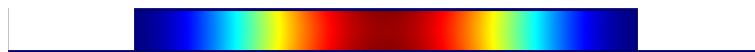
Figure 7.6: Optical mode profile in a double-metal Si waveguide. The substrate has been replaced by a second metallic contact at the bottom of the figure. Adapted from joint publication with C. A. Evans[18].
