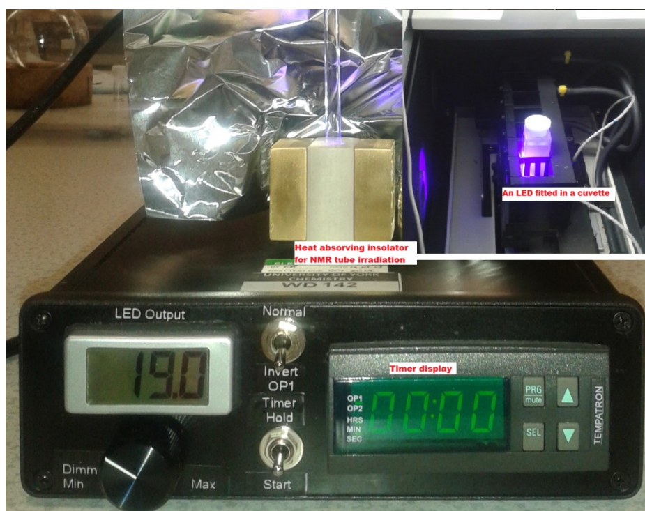
Figure 60 An irradiation system using the 400 nm 5W LED drawing a current of 20 mA
