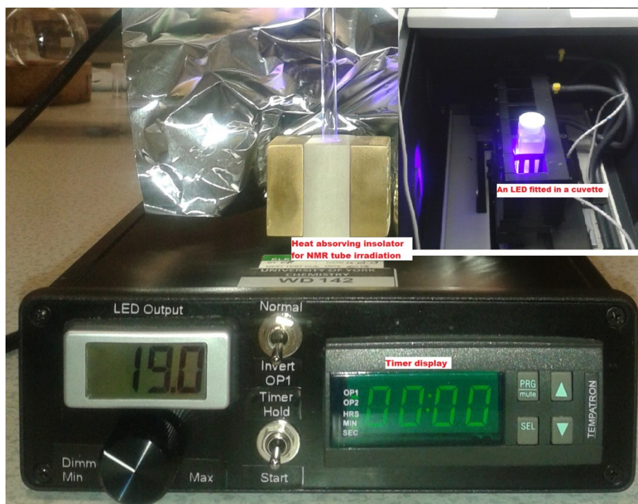
Figure 49 An irradiation system using the 400 nm 5W LED drawing a current of 20 mA.
