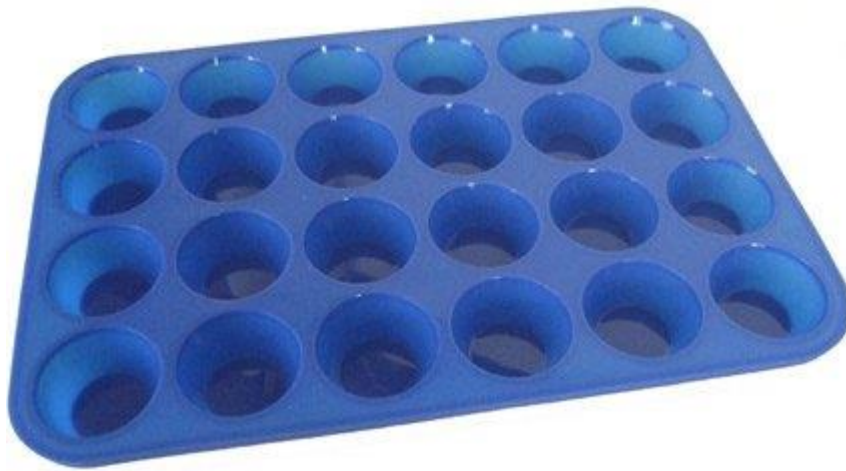
Figure 9. Silicone tray used to cast the shapes of the samples
