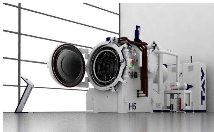
Figure 2.8 Batch sintering furnace (TAV H5) 56
