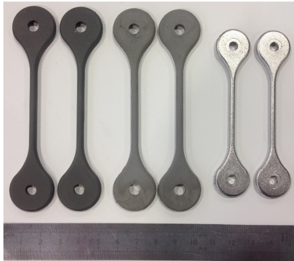
Figure 4.30 Inconel 718 tensile bars for PEG 20000, as moulded (left), debinded (middle) and sintered (right)
