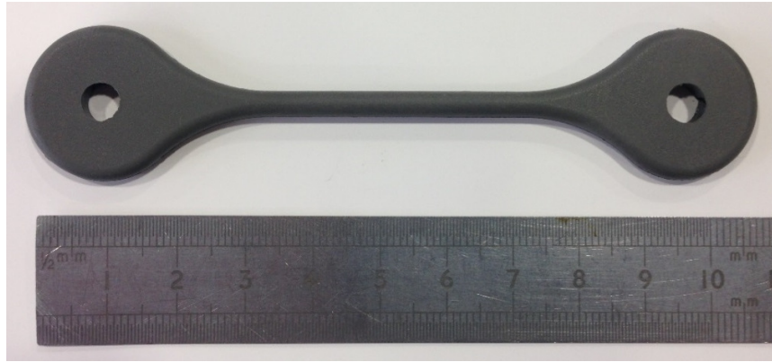
Figure 4.13 Injection moulded tensile bar using PEG 20000
