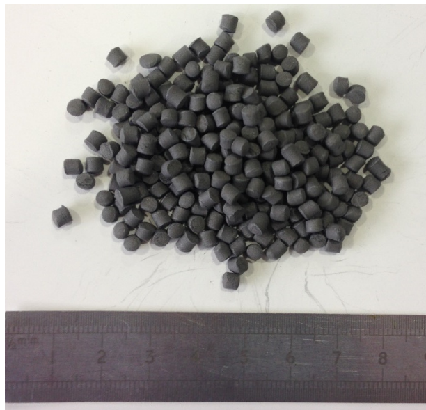
Figure 3.3 Pelletised Inconel 718 feedstock after being extruded twice by the Arburg Injection Moulding Machine, using the Sheffield binder system recipe
