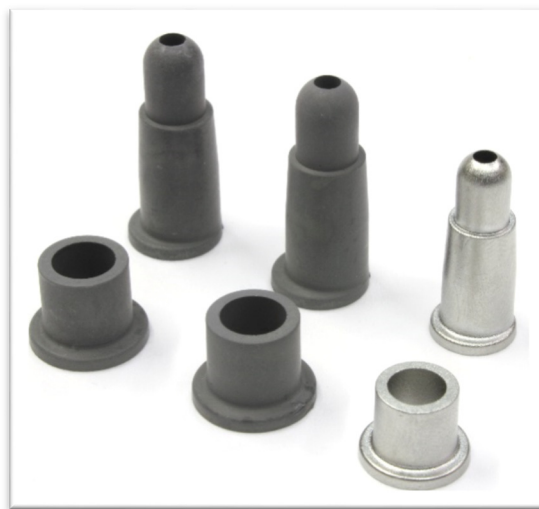
Figure 2.7 Part progression: moulded part (left), debinded part (middle) and sintered part (right) 55 (sintered part height = 25mm)
