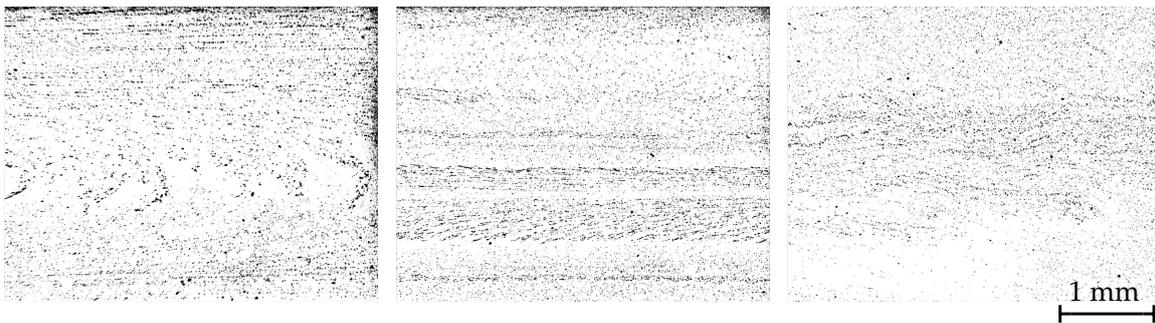
Figure 3.37: Macrostructures of the longitudinal section of the extruded 5 mm diameter CP-Ti wire. Images taken under polarised optical light were converted to binary format to highlight the flow profiles.
