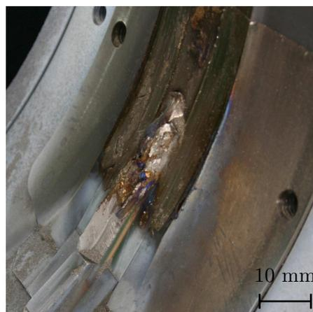
Figure 3.13: The die chamber at the end of Trial 2 showing the fracture surface of the failed abutment with partially consolidated titanium processed over the top.
