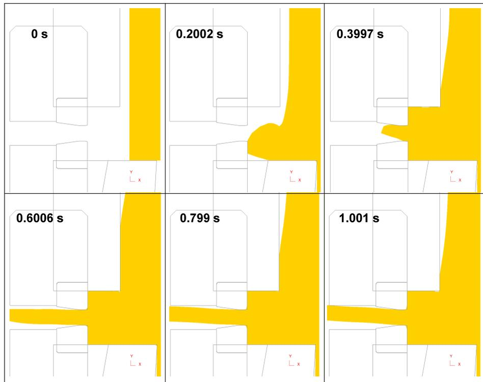
Figure 5.5: Representative finite element simulation in 2D with frames taken at  $\sim 0.2$  second intervals showing the evolution of the upset height during the establishment of steady state Conform extrusion of grade 2 titanium. Maximum upset height and abutment load is achieved at  $t = 0.6$  s.
