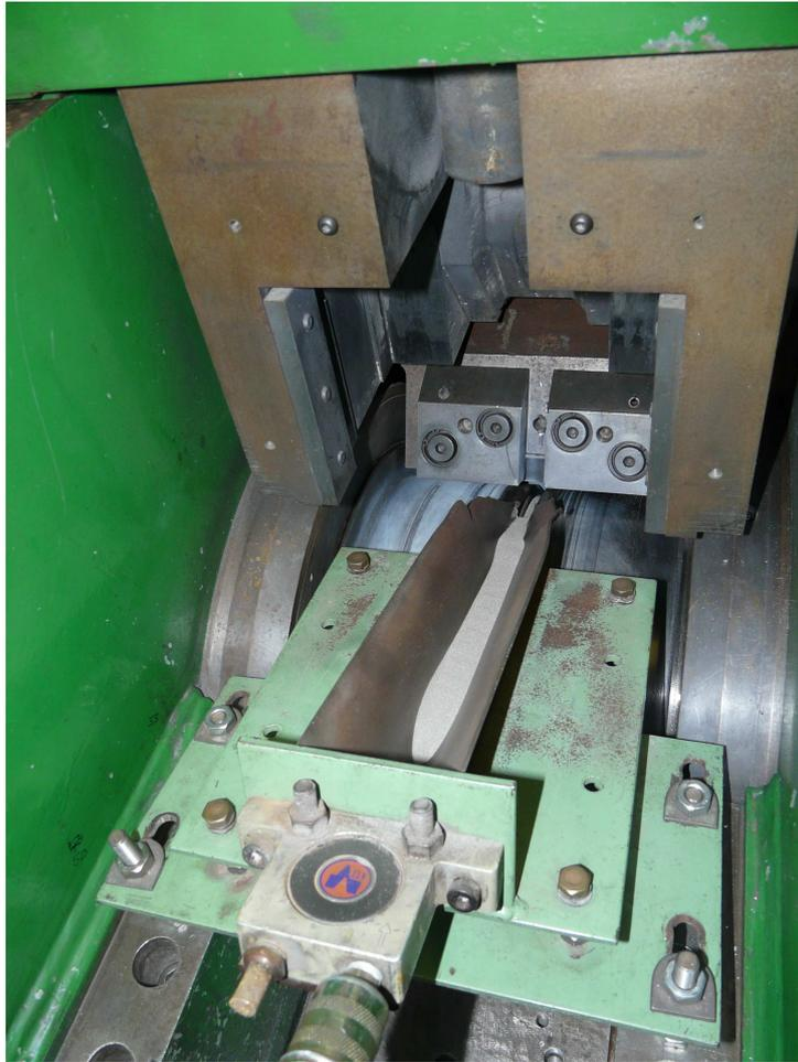
Figure 3.3: Vibrating chute with powder flowing across it and into the wheel groove during an experimental trial.
