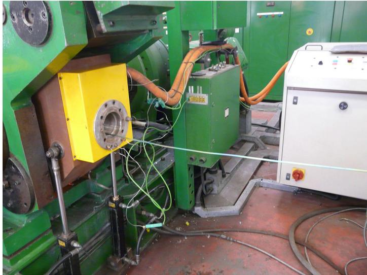
Figure 3.30: 5 mm diameter CP-Ti wire emerging from the BWE Conform<sup>TM</sup> machine before entering a water trough to be quenched.
