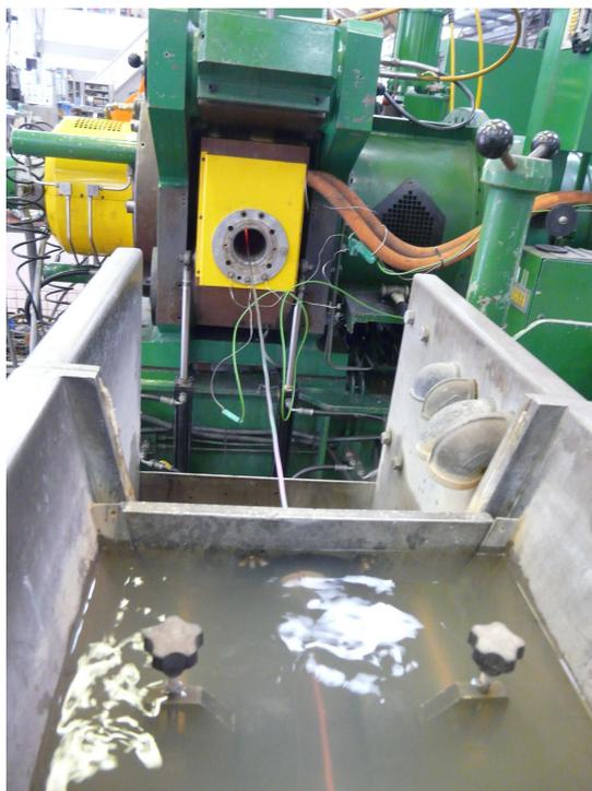
Figure 3.29: 5 mm diameter CP-Ti wire emerging from the BWE Conform<sup>TM</sup> machine before entering a water trough to be quenched.
