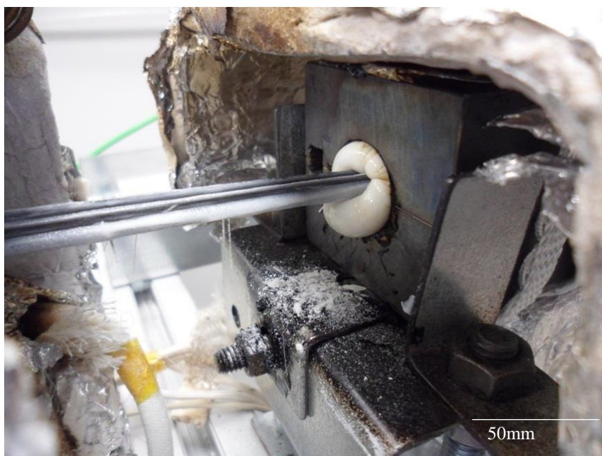
Figure 3.5 Excess polymer building up at the die entrance.
