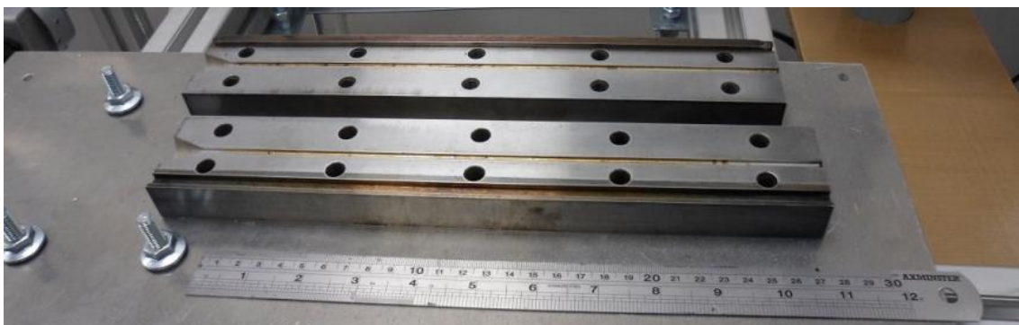
Figure 2.18 Split die halves.
