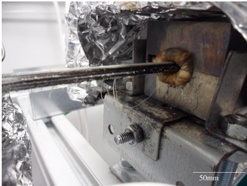
Figure 3.4 If not removed, excess polymer at the die entrance would degrade and block the die, causing the tows to seize at the entrance.
