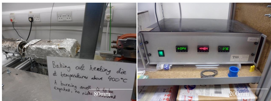
Figure A.17 Annealing of heated die.
