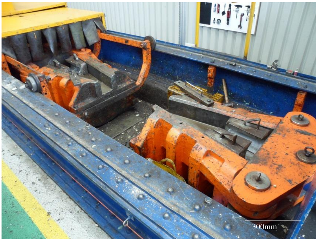
Figure 4.11 Horizontal tensile tester.
