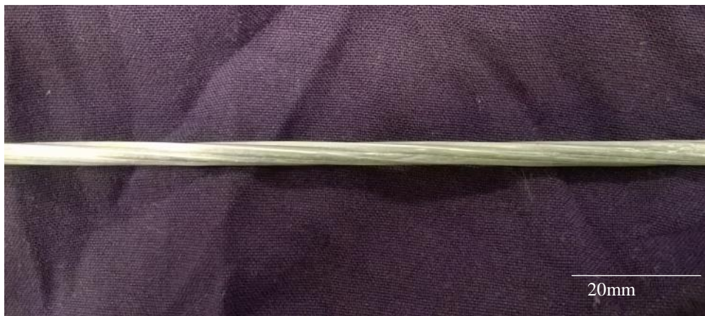
Figure 5.39 Helical pattern indented into shrink wrap tubing surrounding FRP rod.
