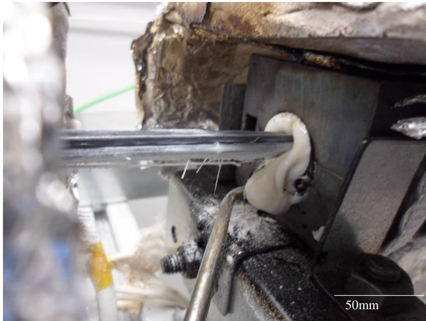
Figure 3.6 Extraction of molten polymer using a machinist's scribe.
