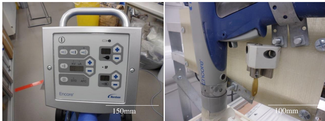
Figure A.13 Manual control of electrostatic spray gun.
