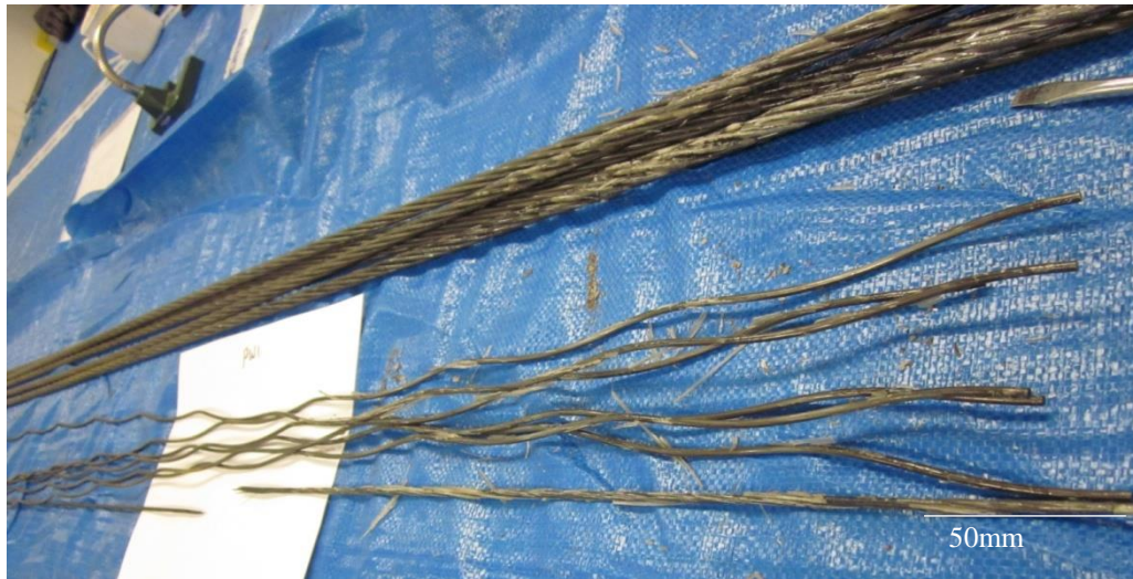
Figure 5.38 Dismantled hybrid strand after testing.
