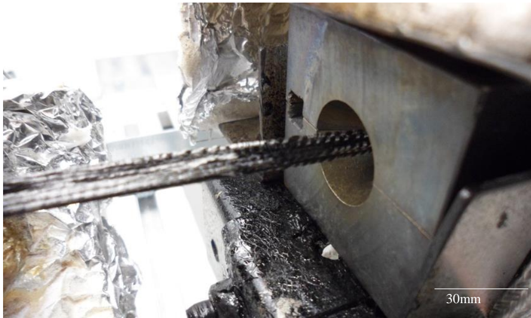
Figure 3.7 Pultrusion of bare commingled tows did not result in a build-up of polymer at the die entrance, which indicated an inadequate quantity of polymer.
