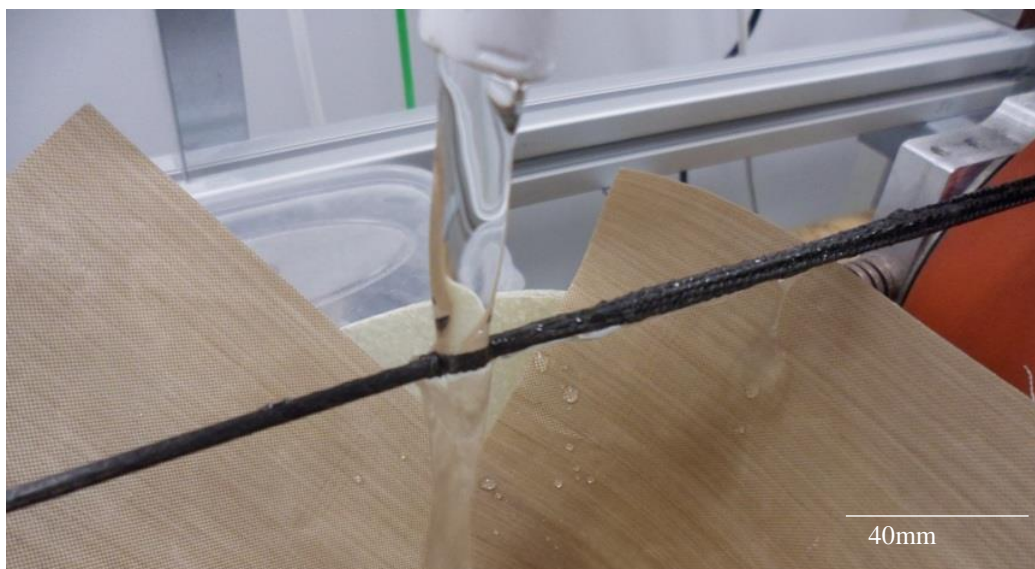
Figure 3.8 A non-circular rod of fused commingled tows emerging from the heating die.
