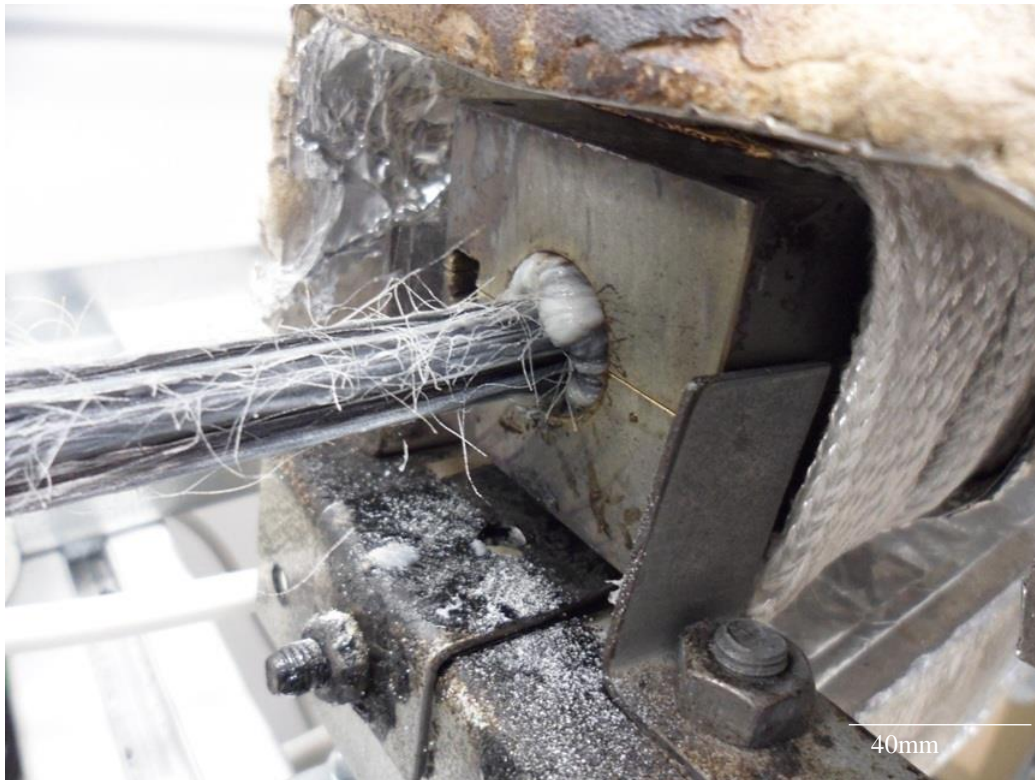
Figure 3.13 Die seizure due to the discontinuities in unsized fibres.
