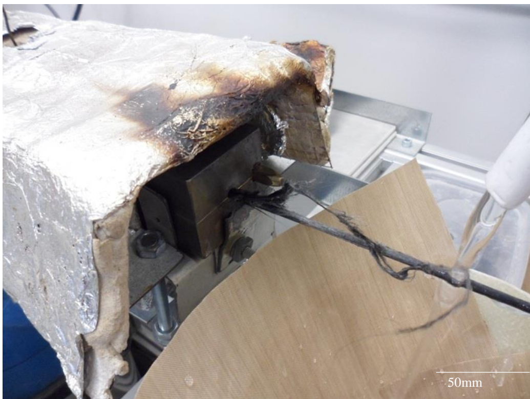
Figure 3.14 Matted fibres emerged from the die after loose fibres were caught at the entrance.
