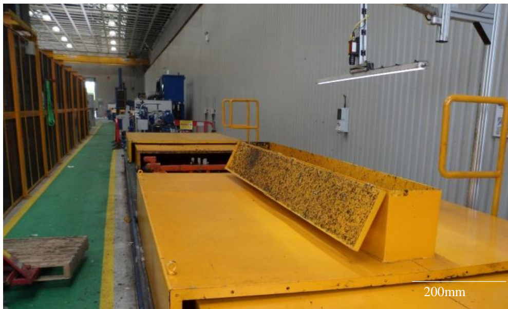
Figure 4.13 Safety covers rolled into place during testing, with an aperture above the test area for the video extensometer and overhead lighting.
