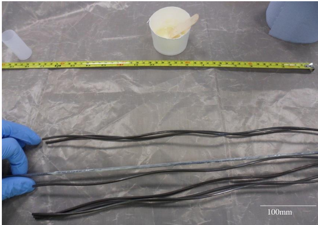
Figure 4.9 Application of Araldite 2011 epoxy adhesive to the far ends of the strand, which were clamped within the testing grips.
