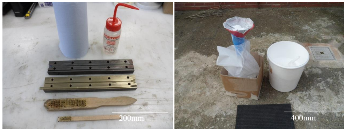
Figure A.20 Scrubbing die with acetone and filtering nylon 12.
