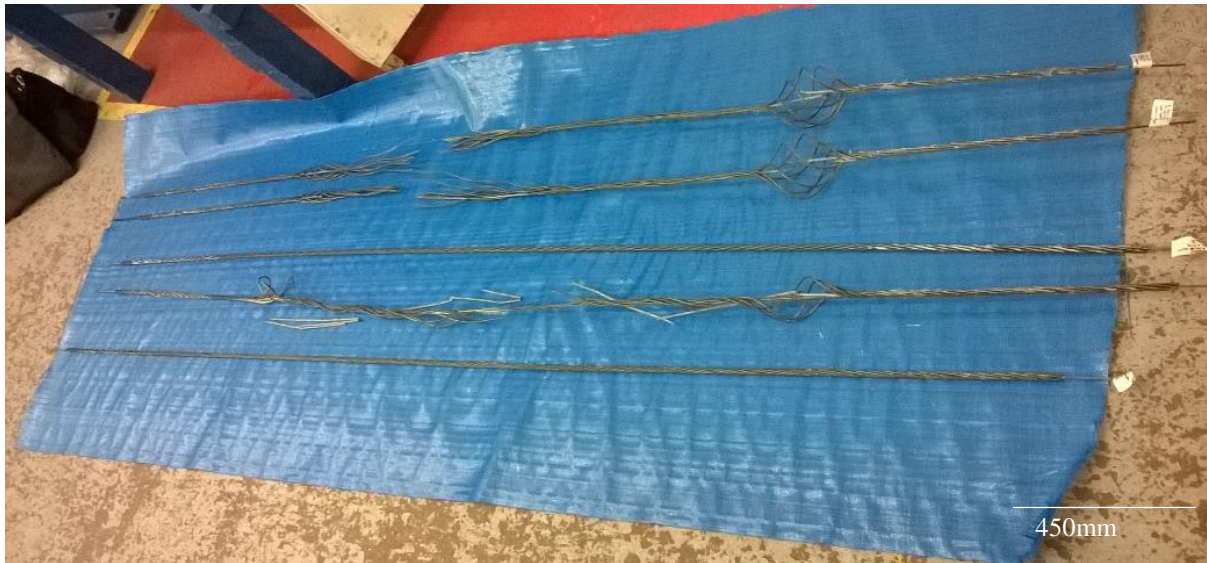
Figure 5.36 Hybrid strands with 6S after testing.
