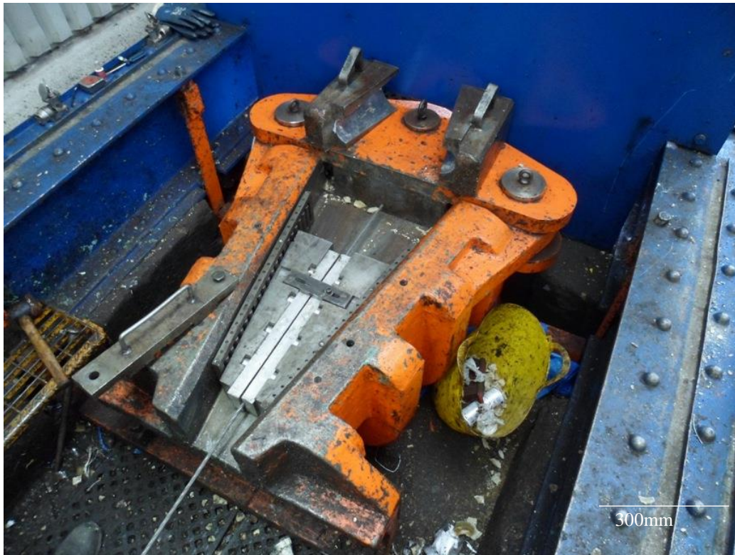
Figure 4.12 Specialised wedge grips with rollers.
