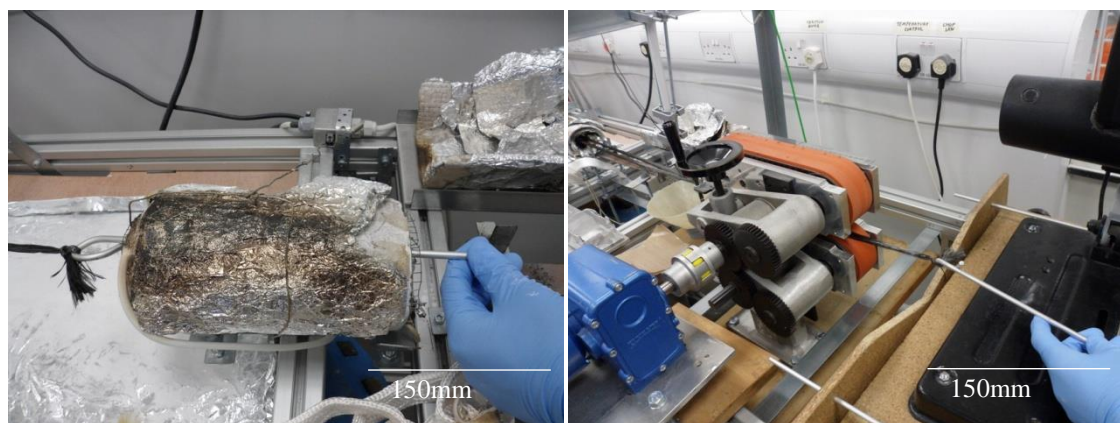
Figure A.5 Pulling tows through pre-heater and traction puller.
