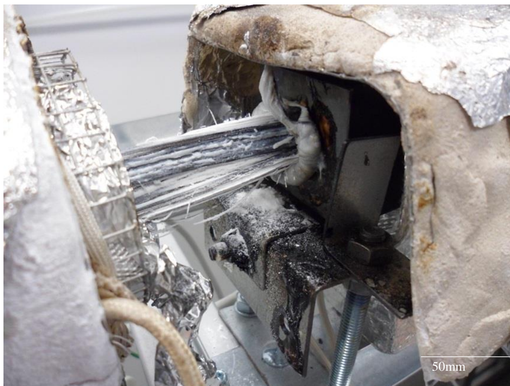
Figure 3.10 Die seizure during attempt to pultrude 5 tows of unsized fibres.
