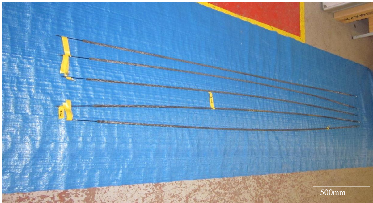
Figure 5.37 Hybrid strands with VE after testing.
