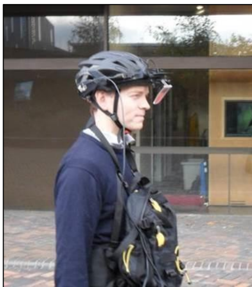
Figure 4.1. SMI iView X HED mobile eye-tracker. Cameras attached to helmet are connected via cables to laptop, carried in rucksack.
