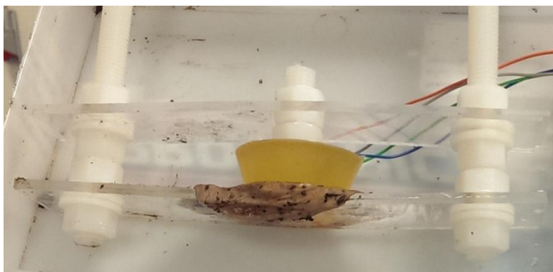
Figure 7.9: Multiple reference resistance characterisation validation test configuration for ex vivo porcine rectal tissue.
