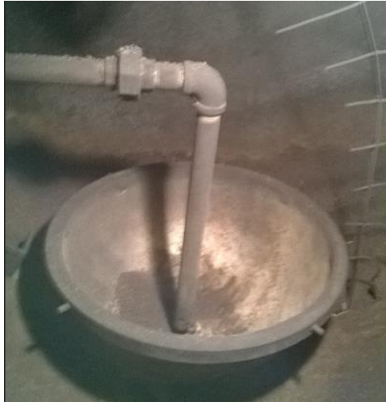
Fig 3.48 Disperser made from dispersion cup design
