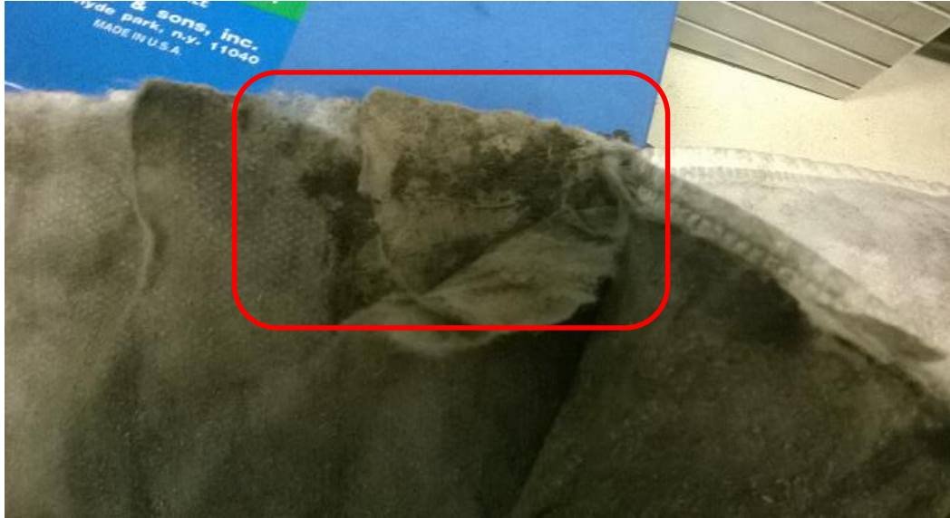
Fig 3.2 Material trapped between the bag layers.
