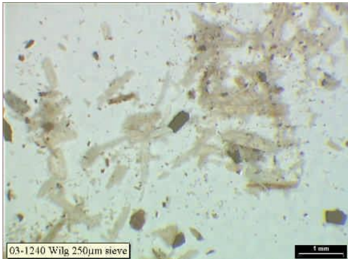
Fig. 2.4 Fresh willow milled in the cutting mill with bottom sieve of 250µm (Bergman, 2011).
