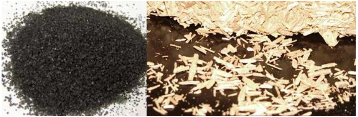
Fig 1.1 Particle shape and size differences between coal dust and woody biomass (Laddha, Zink-Sharp, 1997).
