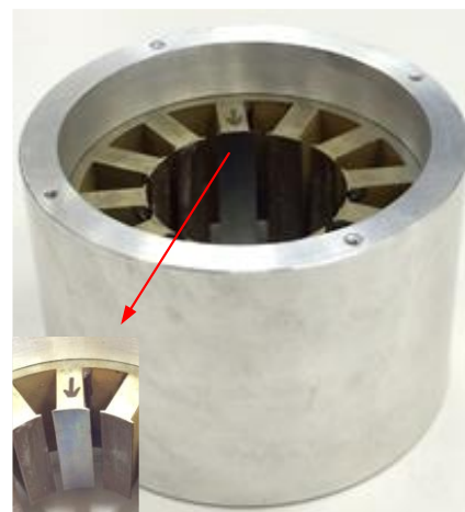
(b) Stator (one 0.2mm tooth-bulge)
