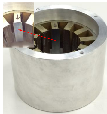
(b) Stator with one tooth-bulge
