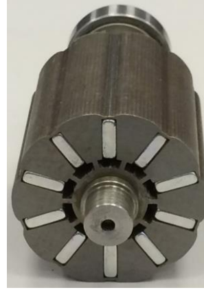
(b) Rotor with conventional airspace barriers
