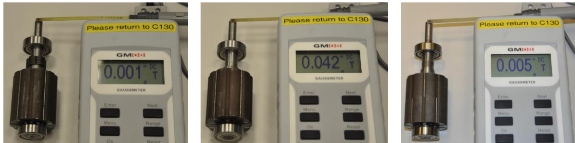
(a) Rotor with conventional airspace barriers (b) Rotor with alternate airspace barriers (c) Step-staggered rotor with alternate airspace barriers.
