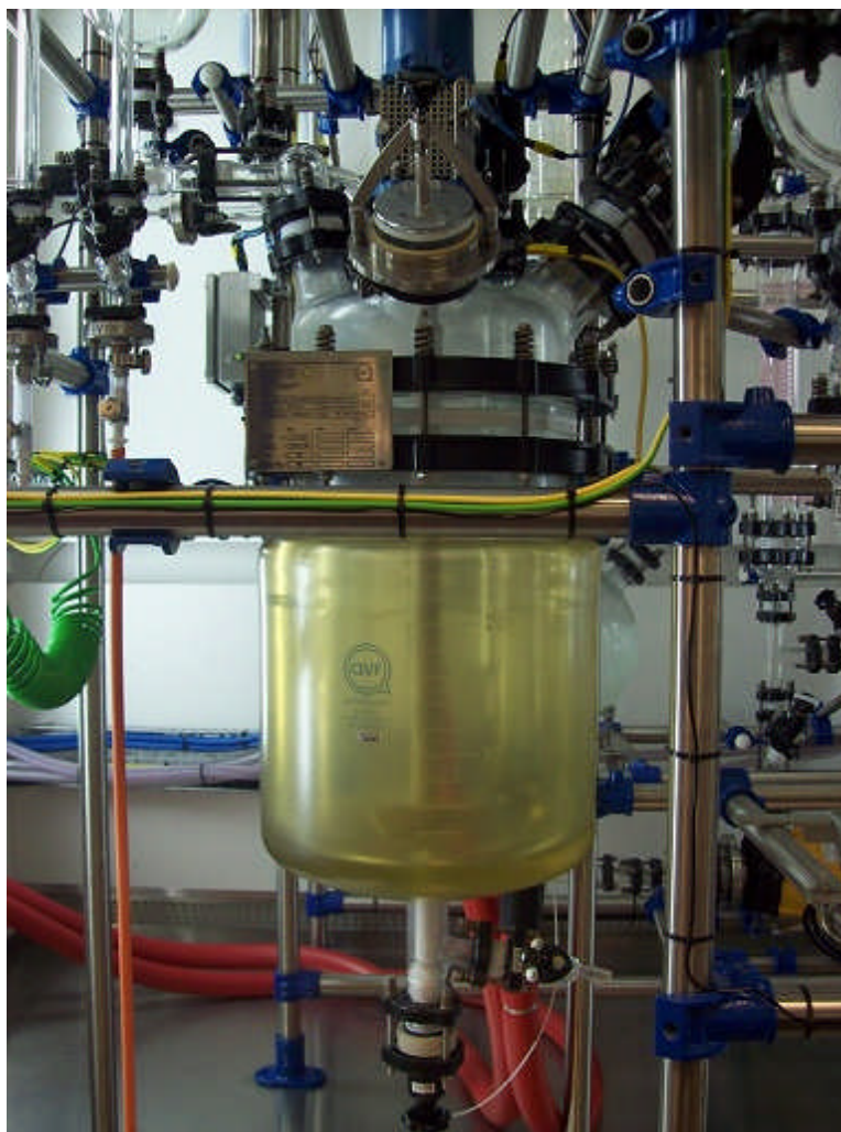
Figure 3.1 – 25 litre jacketed stirred tank reactor, in iPRD, University of Leeds.
