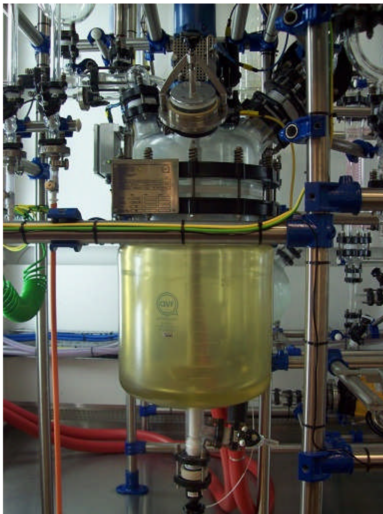
Figure 1.1 – 25 litre jacketed stirred tank reactor in iPRD, University of Leeds.
