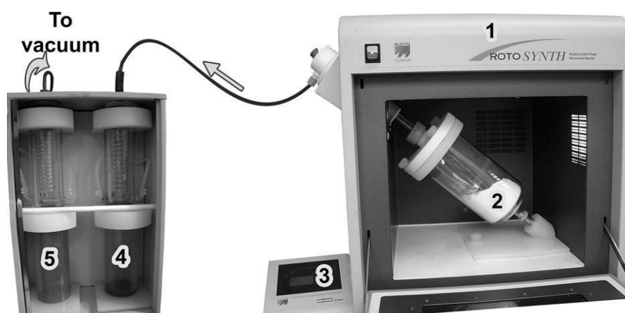
Fig. 1. Schematic of microwave set-up for collection of liquid fractions. (1) Microwave reactor, (2) sample vessel, (3) system control and monitoring console, (4) water cooled condenser for collection of organic fraction and (5) vacuum condenser for collection of aqueous fraction and low molecular weight components.
