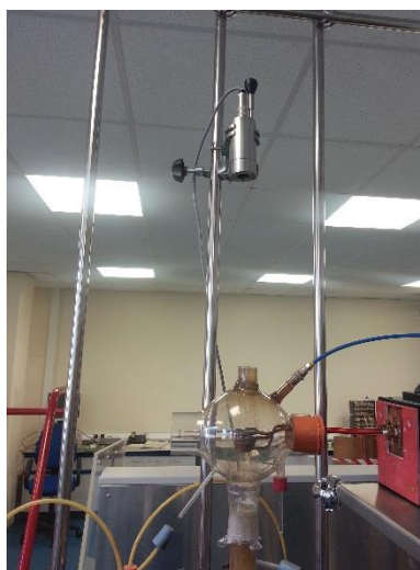
Figure 10: Two-colour pyrometer positioned above levitation chamber and in-line with the middle of the levitation coil
