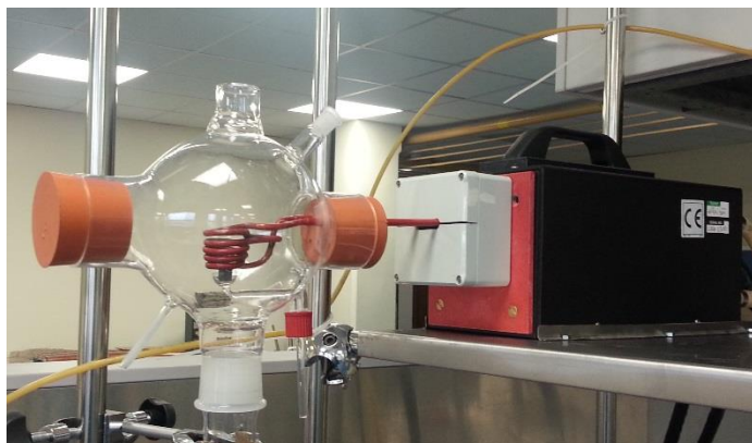
Figure 8: Quartz glass levitation chamber showing various ports for gas flow, coil entry and sample holder
