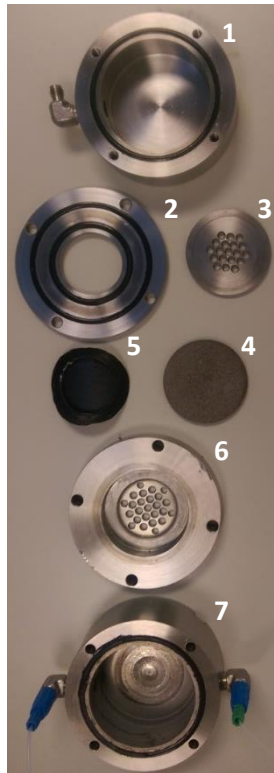
Figure 20 – Pervaporation cell disassembled view
