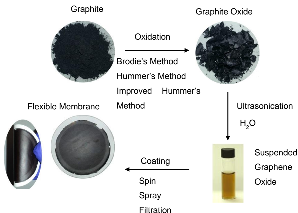
Figure 8 – Overview of the G.O. membrane production process
