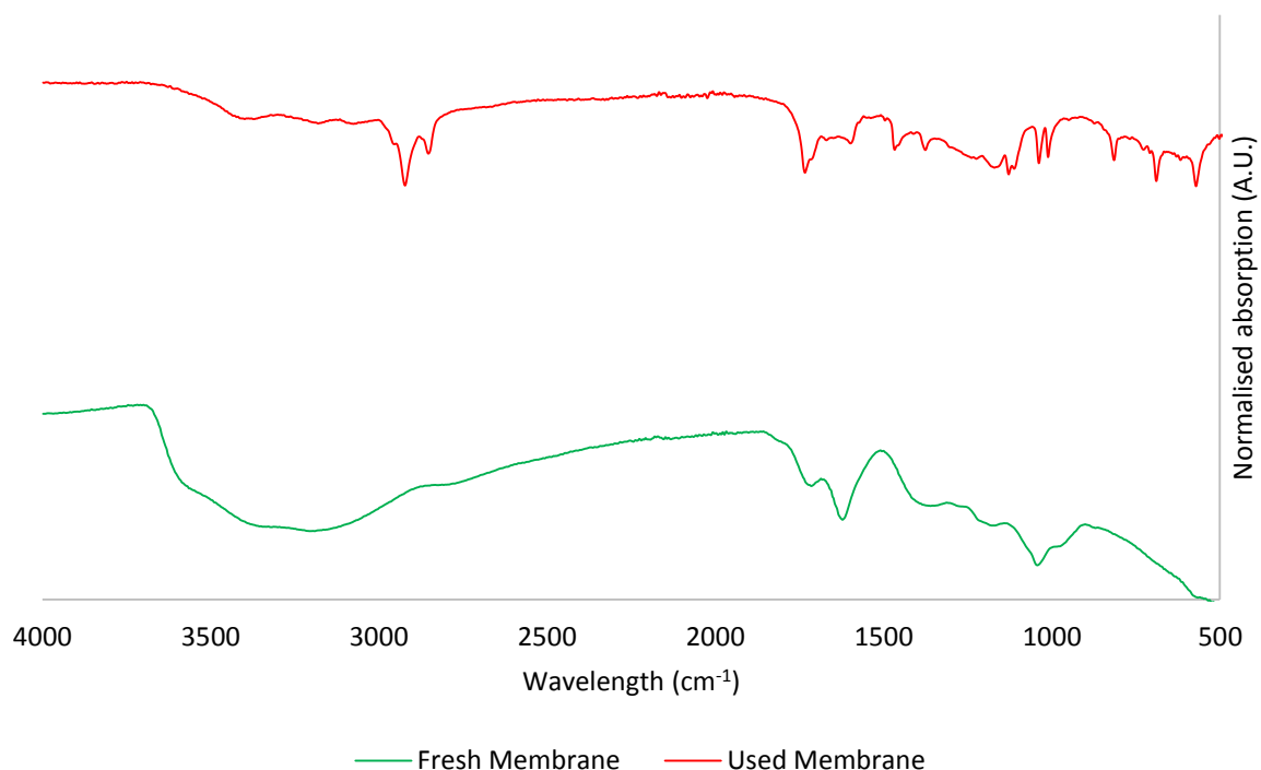
Figure 48-FT-IR spectrum of used (esterification reaction, 100°C, 2.1 \mu\text{m} membrane) and fresh G.O. membrane
