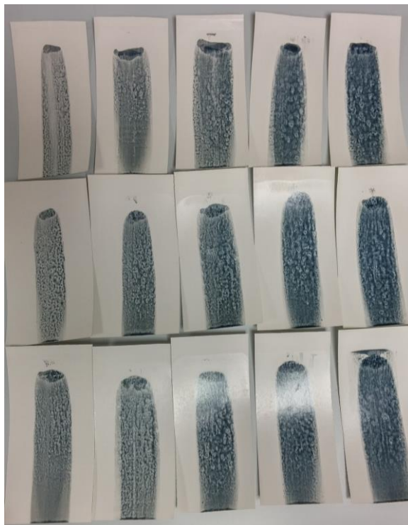
Figure 4.13 Photograph of the PEDOT:PSS coated samples. Samples are numbered 1-15 from top left to bottom right. Increasing number of applications of PEDOT:PSS from one to five layers from left to right in triplicate
