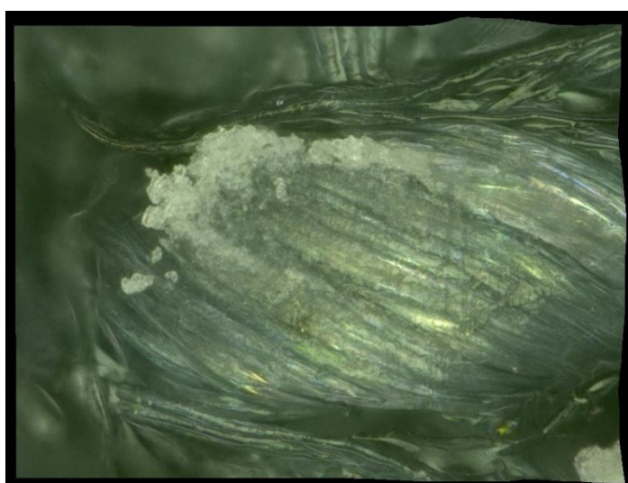
Figure 3.41 3D microscope image of a washed sample treated with four layers of PEDOT:PSS, at 250x magnification
