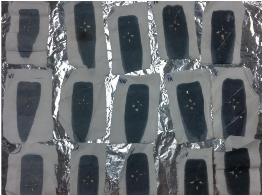
Figure 5.25 An image of the samples after washing and drying. Damage can be seen on a number of samples in the form of creases and even holes.
