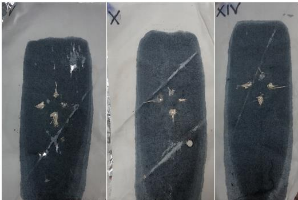
Figure 5.26 Closer inspection of the more damaged samples show the extent of the damage. Electrodes have been removed and the conductive polymer looks to have been removed from the surface by friction.
