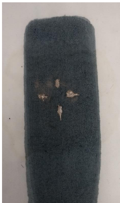
Figure 5.1 Electrically conductive epoxy on the surface of the PEDOT:PSS and latex coated cotton fabric substrate
