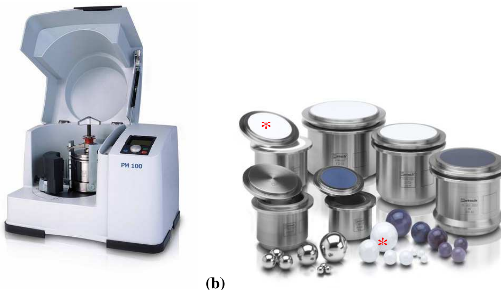
Figure 5.4: Photographs showing (a) Retsch PM100 planetary ball mill and (b) various milling vessels and milling media with the Zirconia milling vessels and milling media used in experiments shown by a red asterisk
