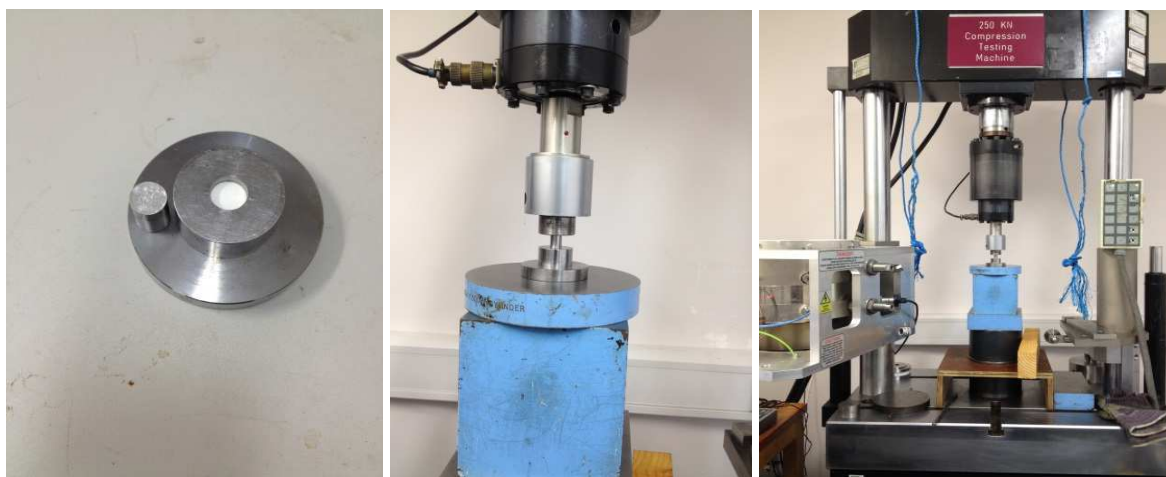
Figure 6.19: Photographs of compression testing experiments showing (a) the die 10 mm filled with \gamma -Al 2 O 3 powder, (b) the 10 mm die on the compression testing machine during loading and (c) a full image of the compression testing machine
