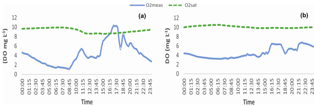
Figure 5.4. Levels of O_{2sat} and O_{2meas} in (a) MHM15 (24 th July), one of only four occasions on which O_{2meas} rose above O_{2sat} and (b) MHM04 (11 th June); an example of the prevalent O_{2meas} / O_{2sat} patterns.
