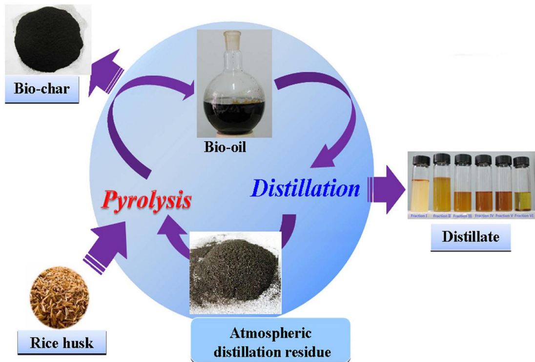
Figure 2- 20 Schematic of the direct atmospheric distillation coupled with co-pyrolysis process to produce chemical feedstock [155]
