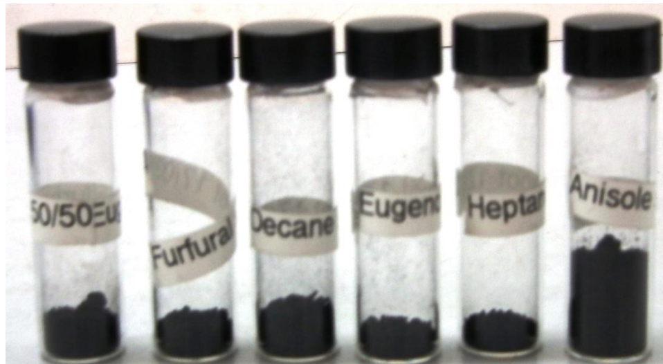
Figure 3-2 Show the soot generated from cold glass slides for analysis
