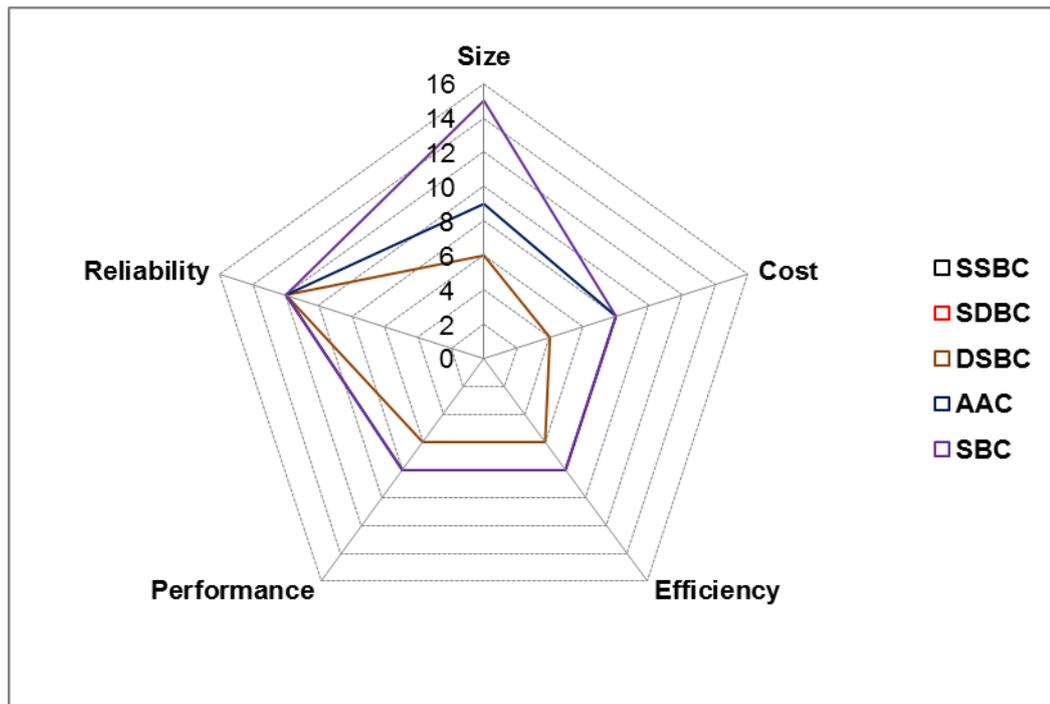
**Figure 2.14: Filled radar showing topology ranking for an offshore power transmission application.**
