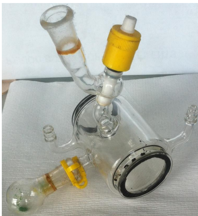
Figure 5.30. The double-walled IR gas cell for used in in-situ vapour/gas release studies.
