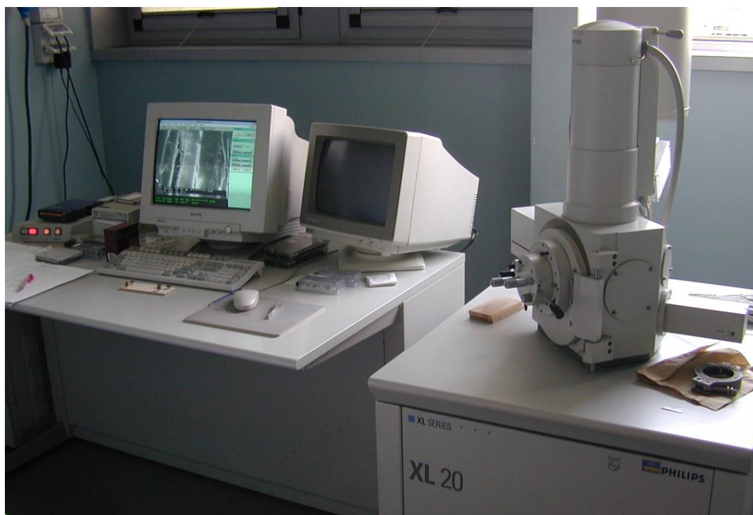
Figure 61: Philips XL20 Scanning Electron Microscope. Operating voltages between 8 and 12 kV, resolution to 4nm and a maximum magnification of x50,000.
