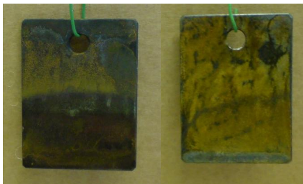
Figure 73: Photograph of A) Mild steel after 24 hrs submersion in 3.5% saline solution and B) mild steel after 1 hr post saline spray, coated with doped PANI (17).
