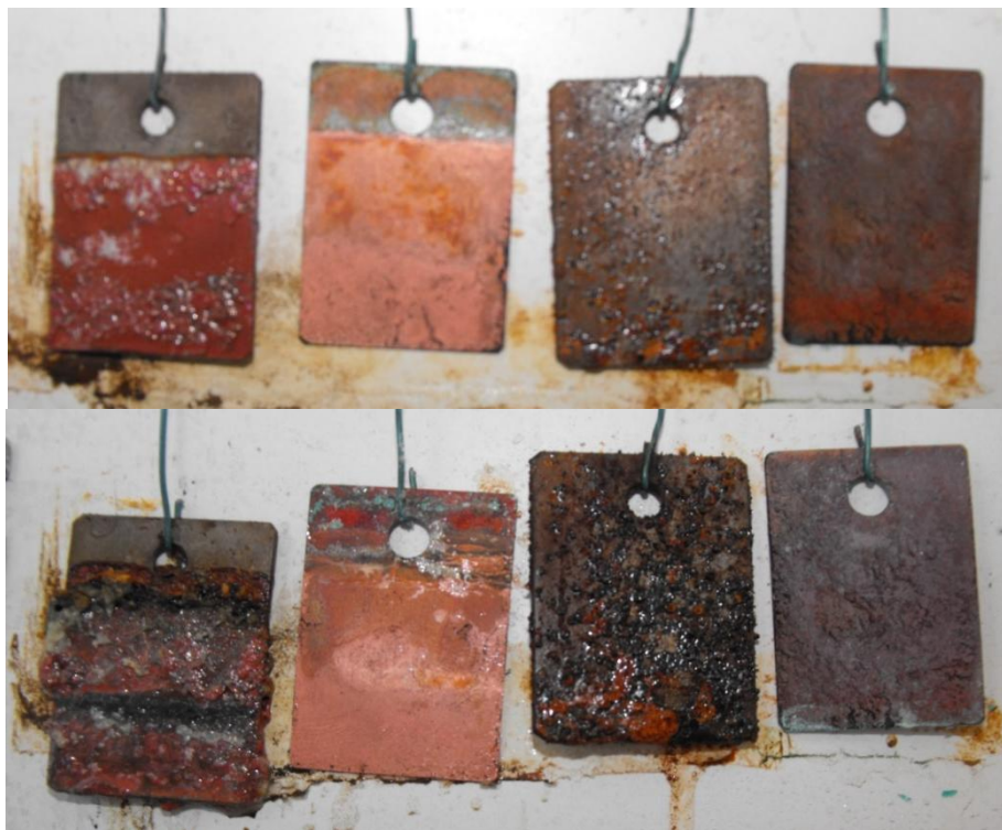
Figure 78: Photograph of both steel and copper 24 hrs of testing (top image) and corrosion noticed after 7 days; from left to right steel submerged, copper submerged, steel sprayed and copper sprayed with (3.5%) saline solution and coated doped PANI (21).
