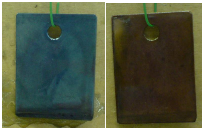
Figure 89: Photographs of steel and copper coated in doped PANI (17) 1 wt% in Epikote 828™, sampled prior to accelerated corrosion testing.
