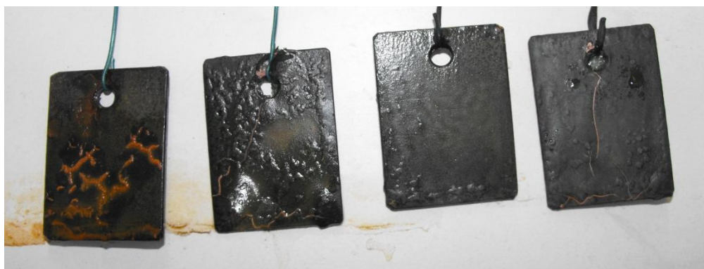
Appendix 17: Photograph of both steel and copper coated with doped PANI (18) 1 wt% in PVC after 7 days (168 hrs) of testing, from left to right; steel submerged, copper submerged in a saline solution (3.5%) and steel sprayed and copper sprayed with (3.5%) saline solution.
