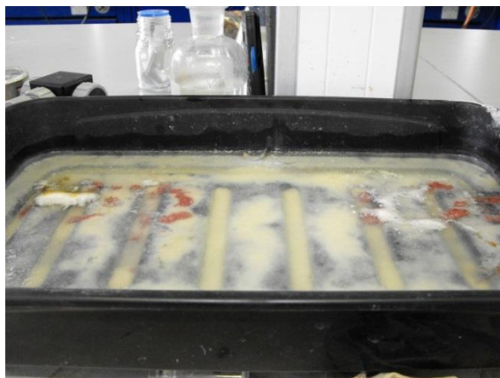
Figure 95: The contamination of the saline solution used in the accelerated corrosion studies; from the reaction of the phosphate doped polymers, the metal substrates and the saline solution.
