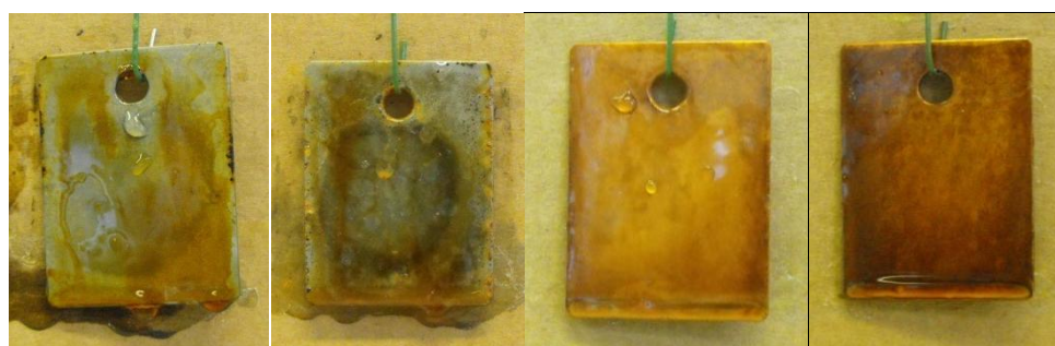
Appendix 12: Metal samples coated in epoxide resin cast films, from left to right; mild steel submerged, mild steel sprayed (3.5% saline), copper submerged and copper sprayed after 7 days incubation.
