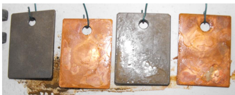
Appendix 13: Metal plates coated in acrylic resin alone prior to accelerated corrosion testing, from left to right; steel then copper for submersion and steel and copper for spraying.
