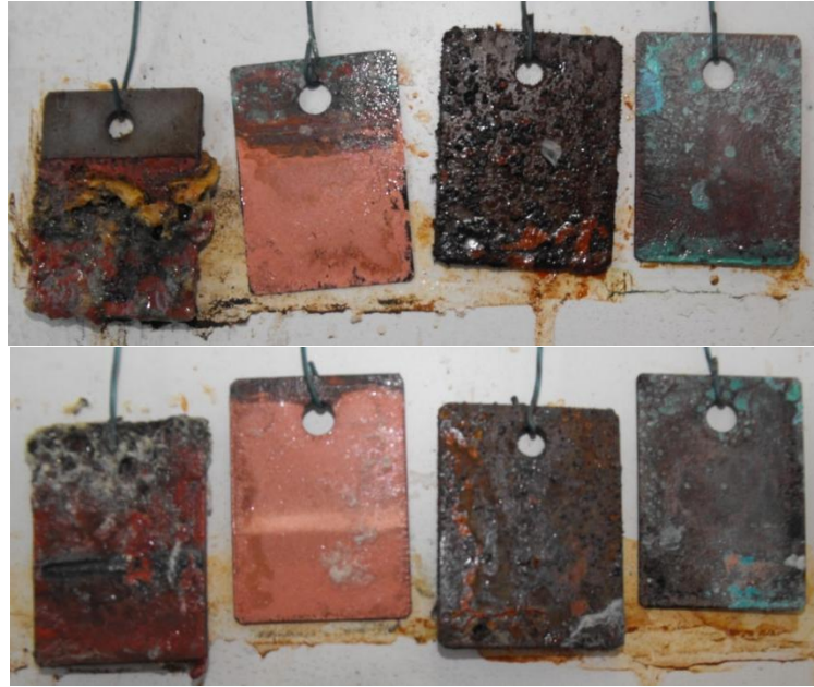
Figure 79: Photograph of both steel and copper 24 hrs of testing (top image) and corrosion noticed after 7 days; from left to right steel submerged, copper submerged, steel sprayed and copper sprayed with (3.5%) saline solution and coated doped PANI (23).
