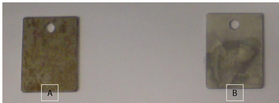
Appendix 9: Photograph of A) Mild Steel before acid pickling and B) After acid pickling.
