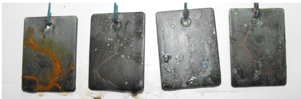
Appendix 18: Photograph of both steel and copper coated with doped PANI (20) 1 wt% in PVC after 7 days (168 hrs) of testing, from left to right; steel submerged, copper submerged in a saline solution (3.5%) and steel sprayed and copper sprayed with (3.5%) saline solution.
