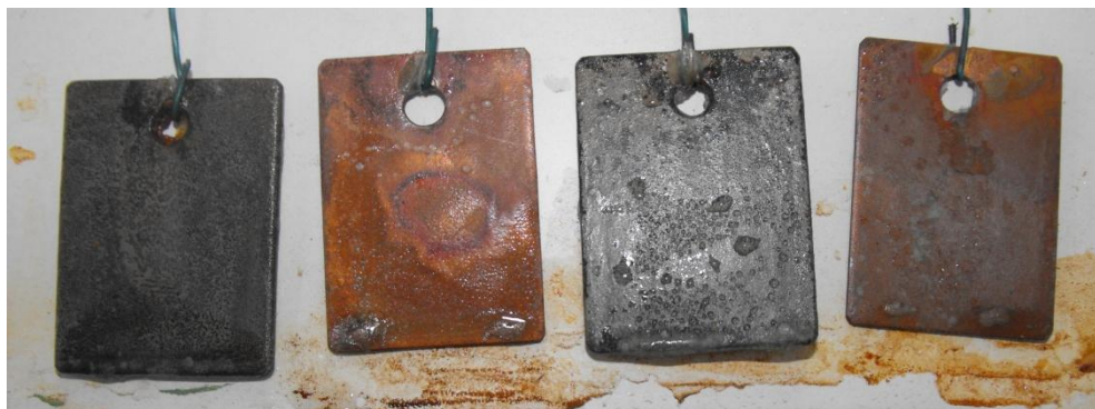
Appendix 21: Photograph of doped PANI ( 21 ) 1 wt% in PVC, dip coated and air dried. From left to right steel submerged, copper submerged in a saline solution (3.5%) after 7 days (168 hrs) and steel sprayed and copper sprayed with (3.5%) saline solution after 7 days (168 hrs).
