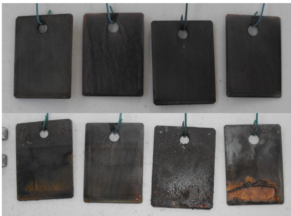
Appendix 15: Photograph of both steel and copper prior to testing (top image) and corrosion noticed after 24hrs; from left to right Steel submerged, copper submerged, steel sprayed and copper sprayed with (3.5%) saline solution and coated doped PANI (18).
