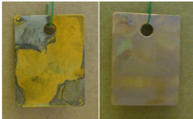
Figure 62: Photograph of mild steel and copper post submersion in a (3.5%) saline solution for 7 days.
