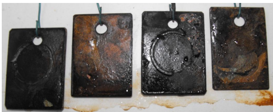
Appendix 23: Photograph of doped PANI ( 18 ) 1 wt% in acrylic resin. From left to right steel submerged, copper submerged in a saline solution (3.5%) and steel sprayed and copper sprayed with (3.5%) saline solution after 7 days (168 hrs).
