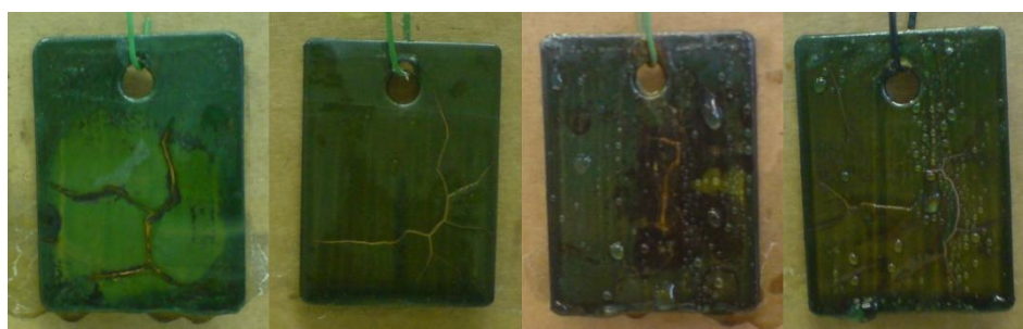
Figure 86: Photograph of doped PANI (17) 1 wt% in PVC, dip coated and air dried. From left to right steel submerged, copper submerged in a saline solution (3.5%) after 120 hrs and steel sprayed and copper sprayed with (3.5%) saline solution after 144 hrs.
