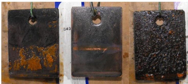
Figure 75: Photograph of both steel and copper submerged for 7 days in (3.5%) saline solution (left and middle image) and effects 7 days after being sprayed with (3.5%) saline solution, coated with doped PANI (22).
