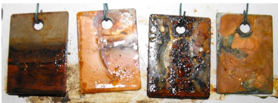
Figure 70: Metal plates coated in acrylic resin alone after 7days (168 hrs) of accelerated corrosion testing. From left to right; steel submerged in brine and copper submerged in brine, steel sprayed with saline and copper sprayed with saline.
