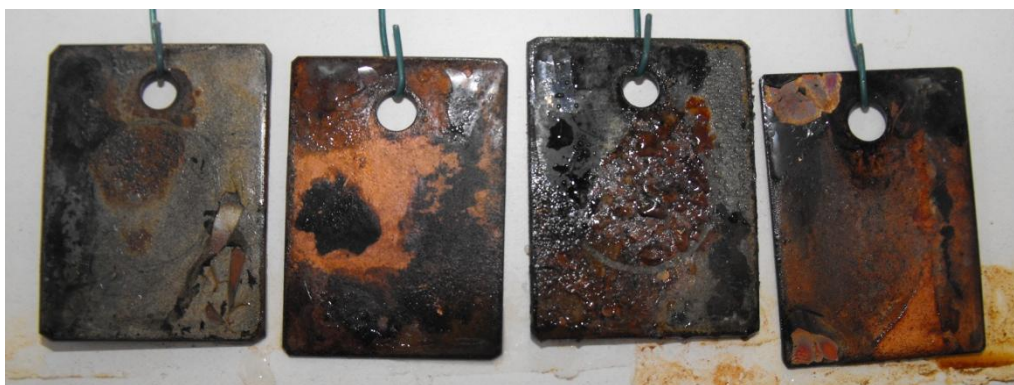
Figure 93: Photograph of doped PANI (20) 1 wt% in acrylic resin. From left to right steel submerged, copper submerged in a saline solution (3.5%) and steel sprayed and copper sprayed with (3.5%) saline solution after 7 days (168 hrs).
