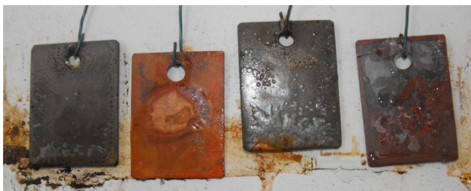
Appendix 22: Photograph of doped PANI ( 23 ) 1 wt% in PVC, dip coated and air dried. From left to right steel submerged, copper submerged in a saline solution (3.5%) after 7 days (168 hrs) and steel sprayed and copper sprayed with (3.5%) saline solution after 7 days (168 hrs).
