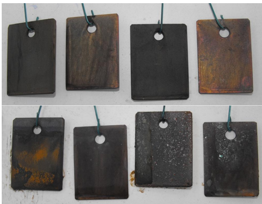
Appendix 16: : Photograph of both steel and copper prior to testing (top image) and corrosion noticed after 24hrs; from left to right steel submerged, copper submerged, steel sprayed and copper sprayed with (3.5%) saline solution and coated doped PANI (20).
