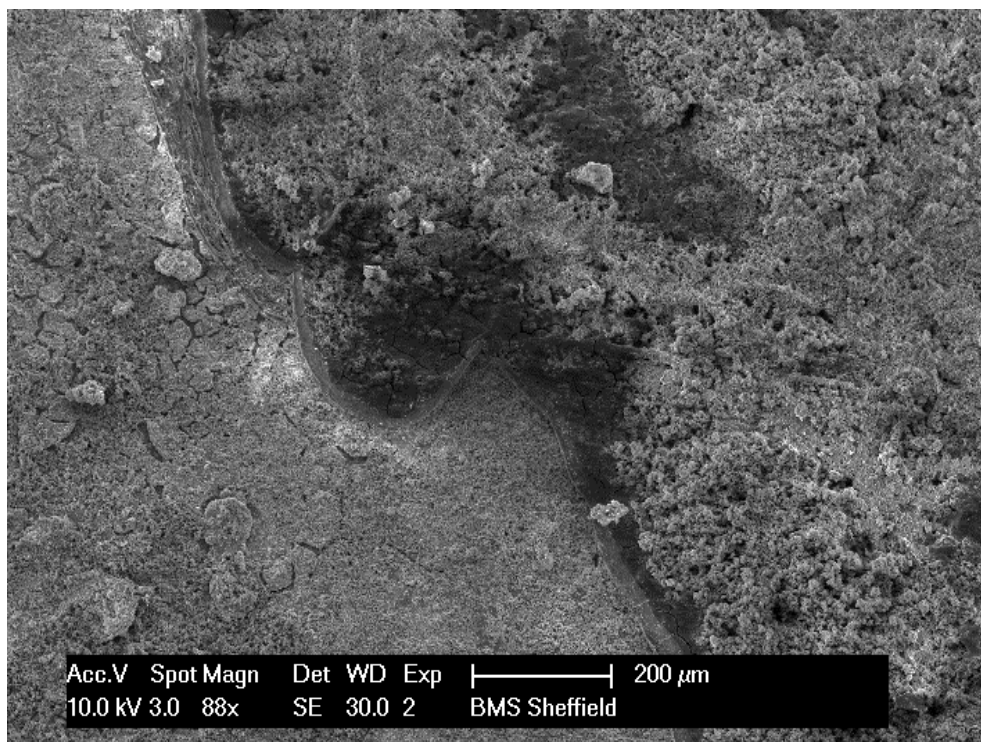
Appendix 27: Steel sample coated with hydroxyl functionalised doped PANI (17). Image shows Polymer (dark area) and Rust (lighter area). Image obtained at 88x magnification.
