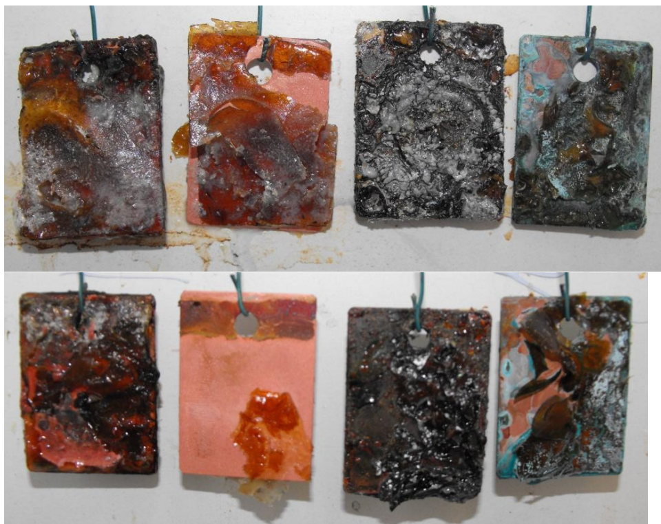
Appendix 24: Photograph of doped PANI (23) 1 wt% in acrylic resin. From left to right steel submerged, copper submerged in a saline solution (3.5%) and steel sprayed and copper sprayed with (3.5%) saline solution after 24 hrs Top image. and after 48 hrs for the bottom image samples.
