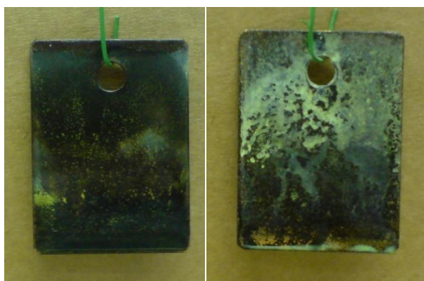
Appendix 14: Photograph of A) Copper after 48 hrs submersion in 3.5% Saline Solution and B) Copper after 1 hr post saline spray Doped PANI (17).
