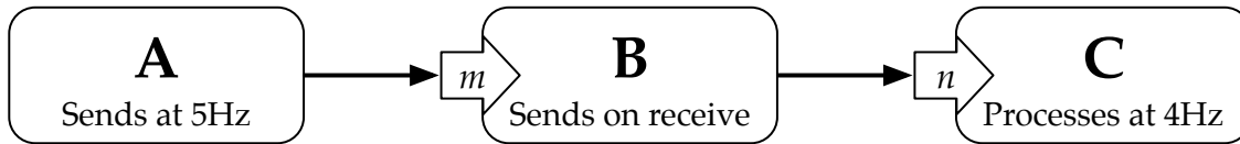
Figure 5.7: An example application with three machines A , B , and C that are formed into a pipeline arrangement. Regardless of B and C 's channel buffer lengths, m and n , messages will always eventually be lost as C cannot process data fast enough and B does not control the rate of data generation.
