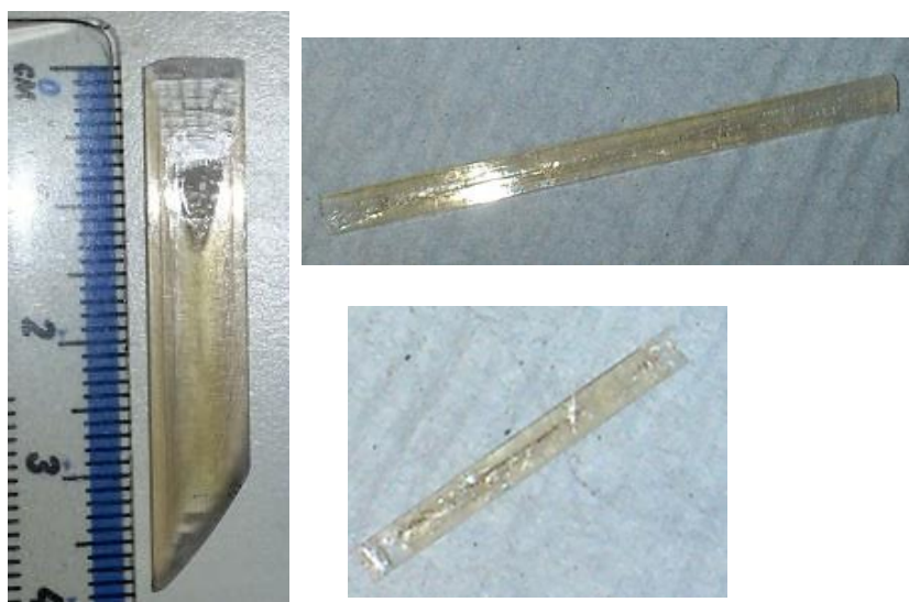
Figure 8-12: \alpha -pABA crystals grown from 90:10 EtOH:NMe solutions by slow solvent evaporation. Crystals took around 3 weeks to appear
