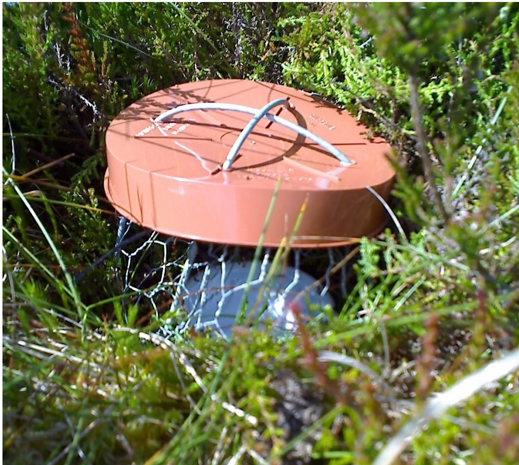
Figure 3.4: A pitfall trap with lid and mesh surround
