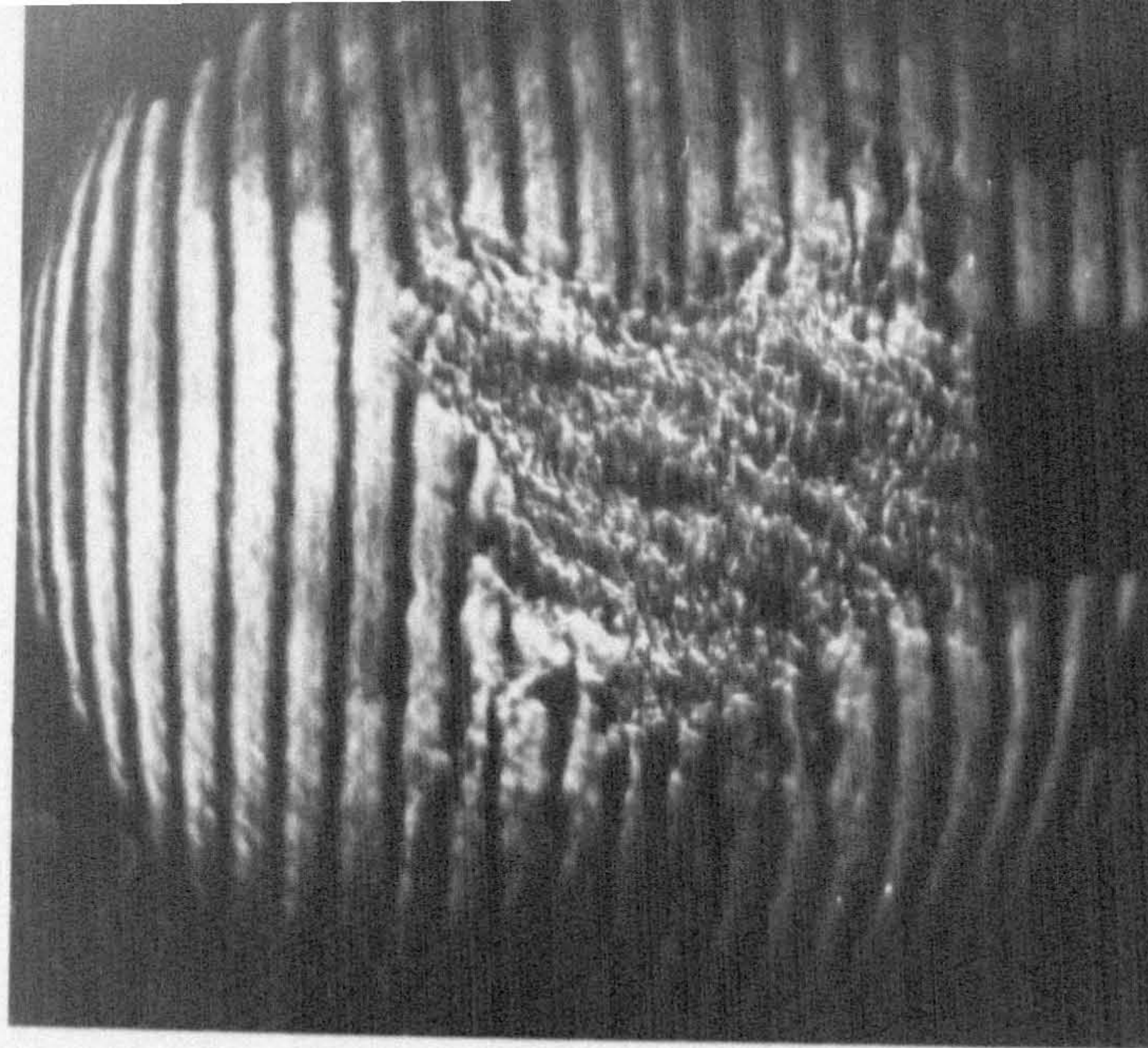
(a) 13.04% CH 4 -AIR 12 J (COMPLETE PROPAGATION)
