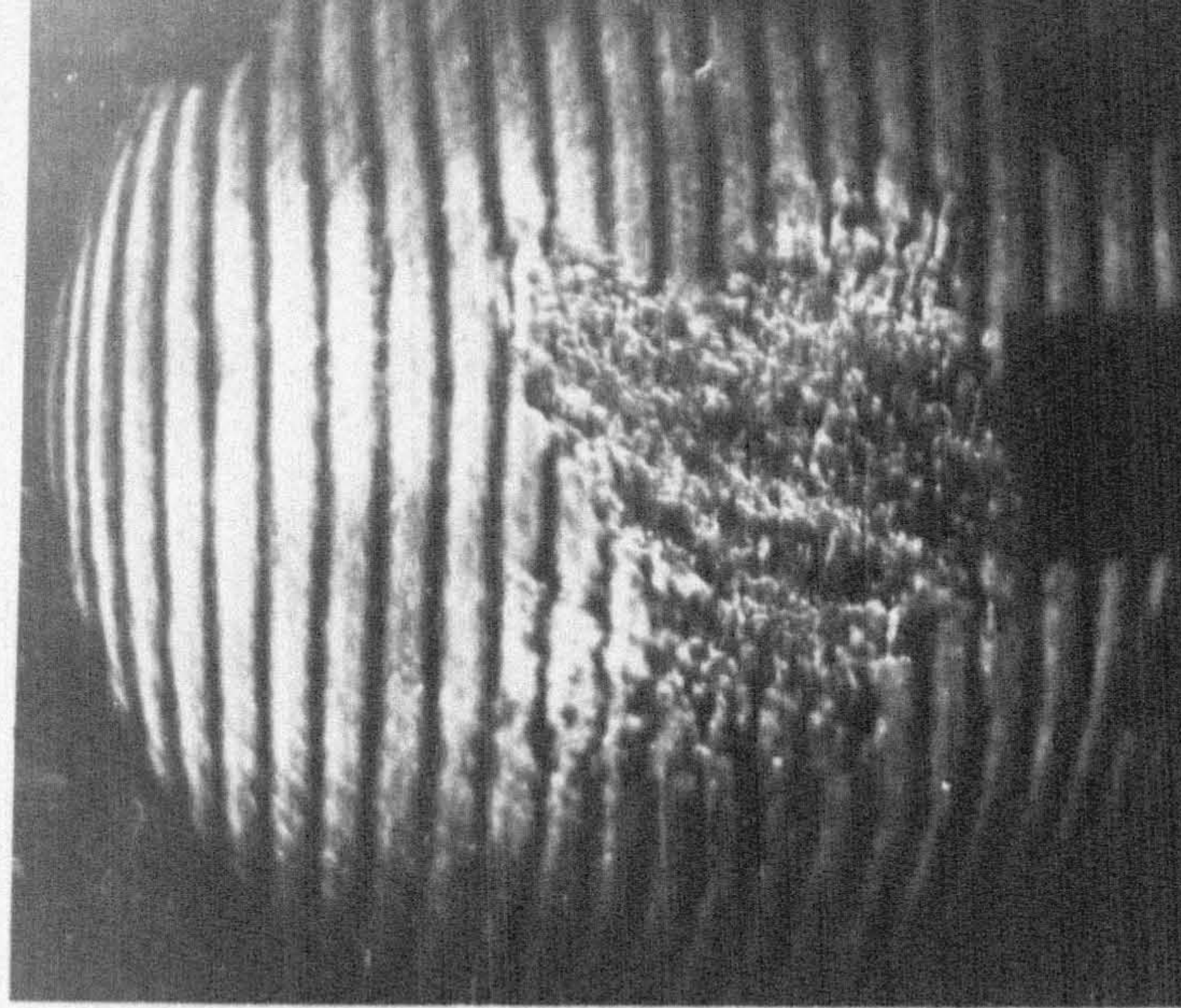
(a) 13.04% CH 4 -AIR 12 J (COMPLETE PROPAGATION)
