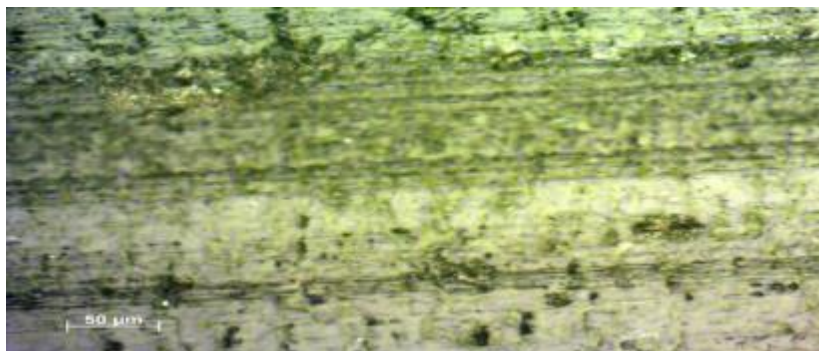
Fig. 24- Contact Surface after 60 Minutes at 3.3 m/sec and 50 N Test.
