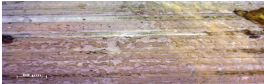
Fig. 154- Contact Surface after 30 Minutes at 3.3 m/sec and 30 N Test.
