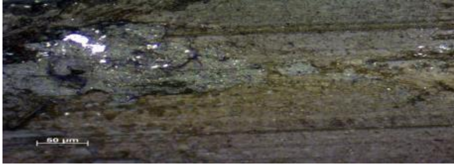
Fig. 145- Contact Surface after 05 Minutes at 1.5 m/sec and 50 N of Test.
