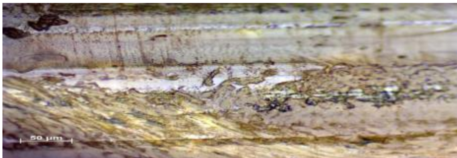
Fig. 147- Contact Surface after 60 Minutes at 1.5 m/sec and 50 N Test.
