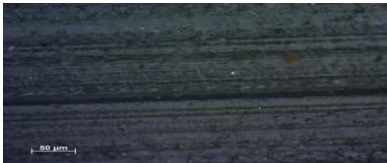
Fig. 8- Contact Surface after 60 Minutes at 1.5 M/sec and 30 N Test.
