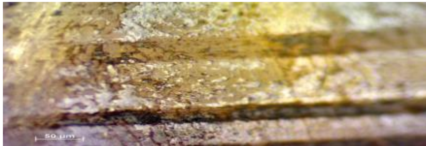
Fig. 159- Contact Surface after 60 Minutes at 3.3 m/sec and 50 N Test.
