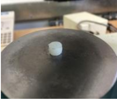
Fig. 8:10- Nylon 66 Material Specimen after Test.
