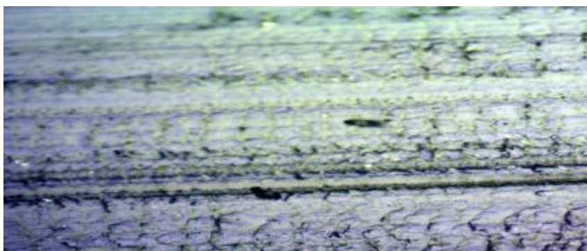
Fig. 44- Contact Surface after 60 Minutes at 1.5 m/sec and 50 N Test.
