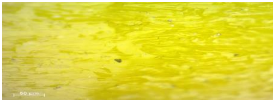
Fig. 99- Contact Surface after 05 Minutes at 7.2 m/sec and 50 N Test.
