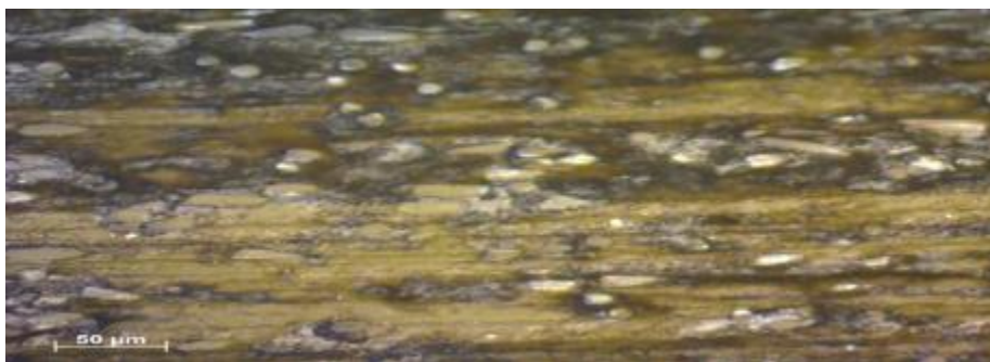
Fig. 83- Contact Surface after 05 Minutes at 3.3 m/sec and 30 N Test.
