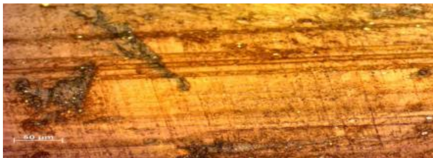
Fig. 138- Contact Surface after 30 Minutes at 1.5 m/sec and 10 N Test.
