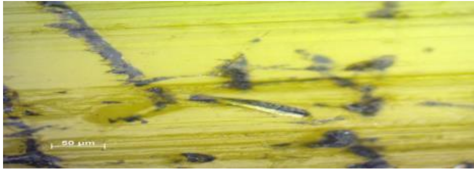
Fig. 69- Contact Surface after 60 Minutes at 1.5 m/sec and 10 N Test.
