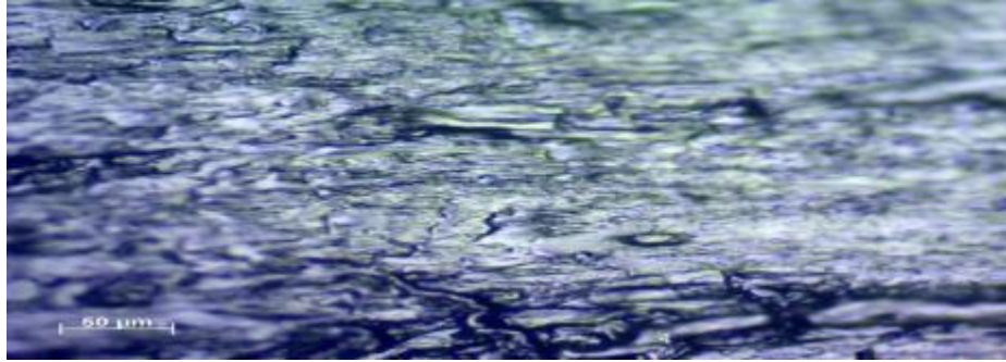
Fig. 65- Contact Surface after 05 Minutes at 7.2 m/sec and 50 N Test.
