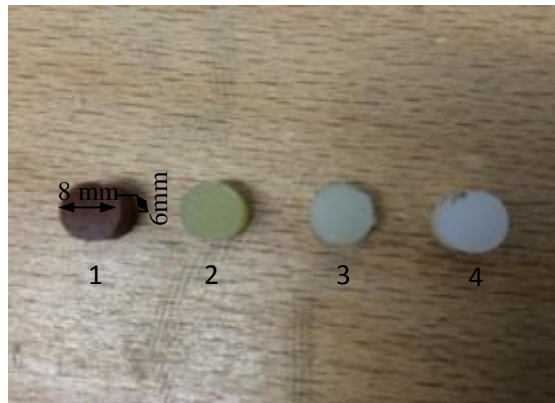
Fig. 8:3- End Post Materials Specimens (1) PRBF, (2) EG, (3) N12, and (4) N66 Materials.
