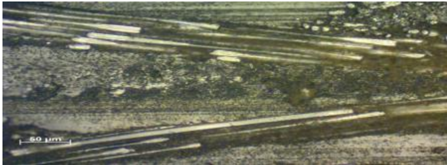
Fig. 110- Contact Surface after 30 Minutes at 1.5 m/sec and 50 N Test.
