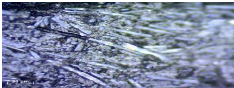
Fig. 96- Contact Surface after 30 Minutes at 7.2 m/sec and 30 N Test.
