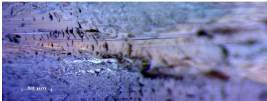
Fig. 170- Contact Surface after 30 Minutes at 7.2 m/sec and 50 N Test.
