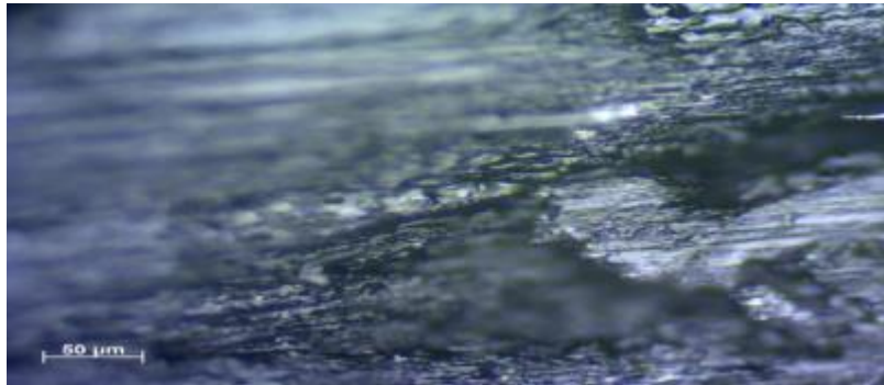
Fig. 30- Contact Surface after 05 Minutes at 7.2 m/sec and 30 N Test.
