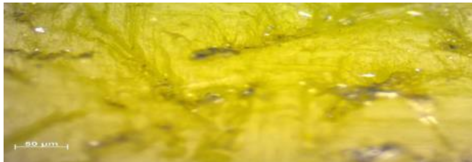
Fig. 67- Contact Surface after 05 Minutes at 1.5 m/sec and 10 N Test.
