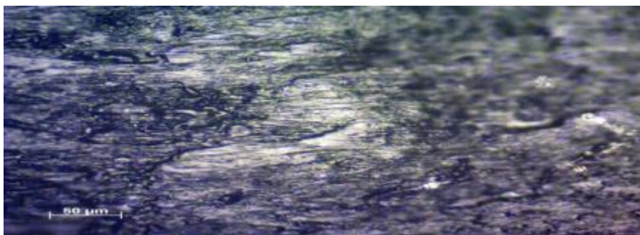
Fig. 52- Contact Surface after 60 Minutes at 3.3 m/sec and 30 N Test.
