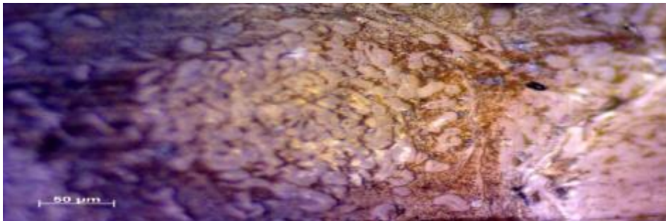
Fig. 151- Contact Surface after 60 Minutes at 3.3 m/sec and 10 N Test.
