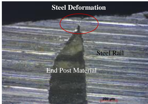
Fig. 6:8- R3 Specimen Imitating Rail Head Deformation over the Insulating End Post (0.5 mm)
