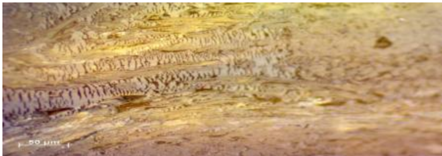
Fig. 163- Contact Surface after 60 Minutes at 7.2 m/sec and 10 N Test.
