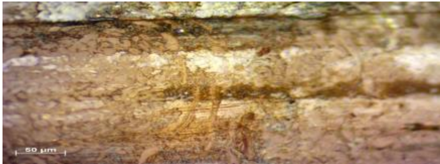
Fig. 158- Contact Surface after 30 Minutes at 3.3 m/sec and 50 N Test.
