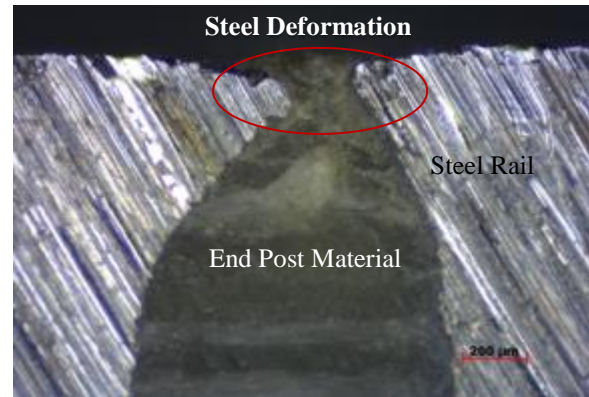
Fig.6:9- R3 Specimen Imitating Rail Head Deformation over the Insulating End Post (1 mm)
