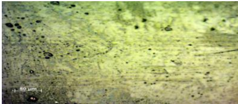
Fig. 22- Contact Surface after 05 Minutes at 3.3 m/sec and 50 N Test.
