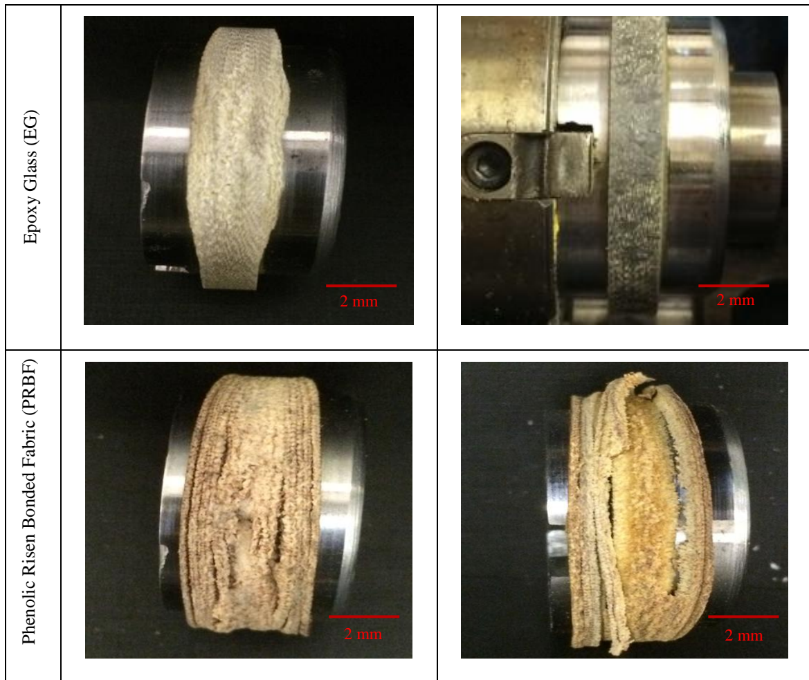
Fig. 7:2- Specimens Tested Surface Images of Nylon 12, Nylon 66, Nylon 66a, Epoxy Glass and Phenolic Resin Bonded Fabric Materials.
