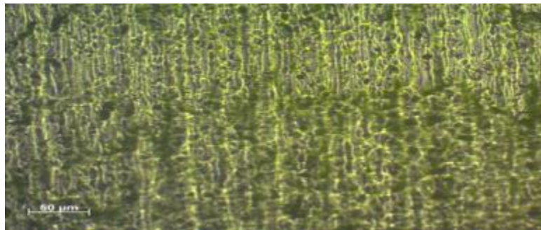
Fig. 6- Contact Surface after 05 Minutes at 1.5 m/sec and 30 N Test.
