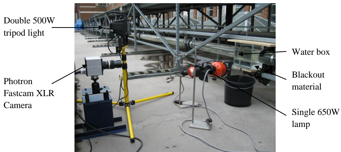
Figure 5 Configuration of the High Speed Image Velocimetry Apparatus
