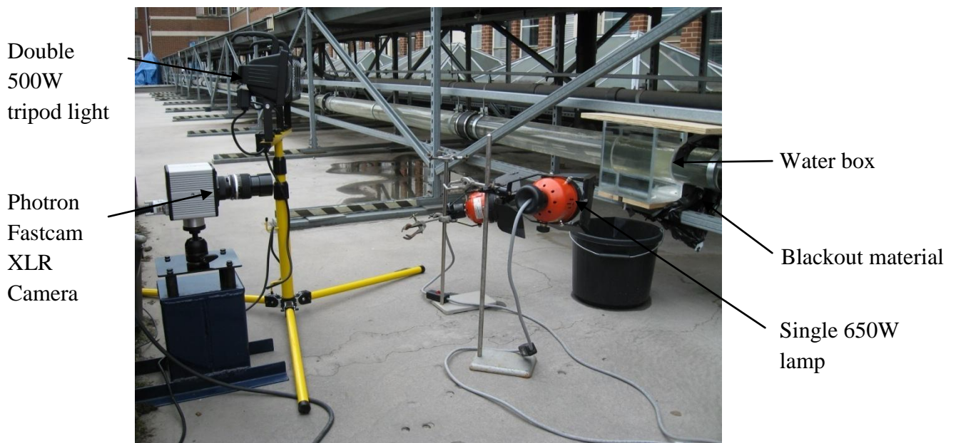
Figure 3.26 Image of the Camera Configuration
