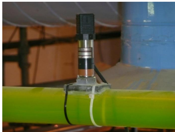
Figure 2.14 Pressure Transducer within the Crown of the Horizontal Carrier Pipe
