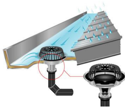
Figure 1.3 Diagram of a Typical Siphonic System (Fullflow Group Ltd (2016) "Syphonic Explained"
