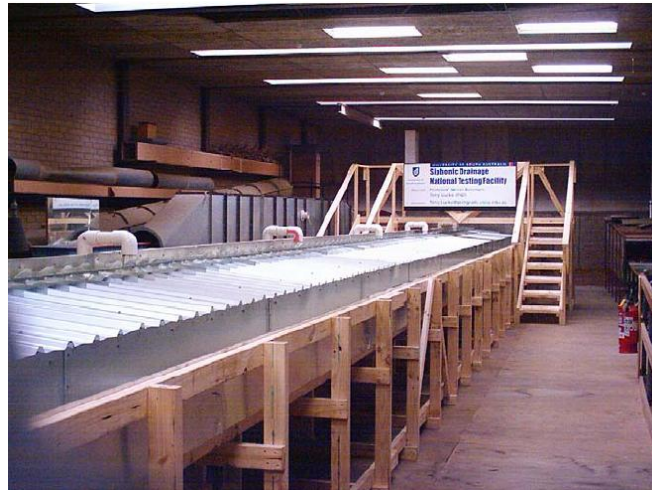
Figure 2.17 The UniSA Siphonic Drainage Test Facility (Lucke et al. 2007)
