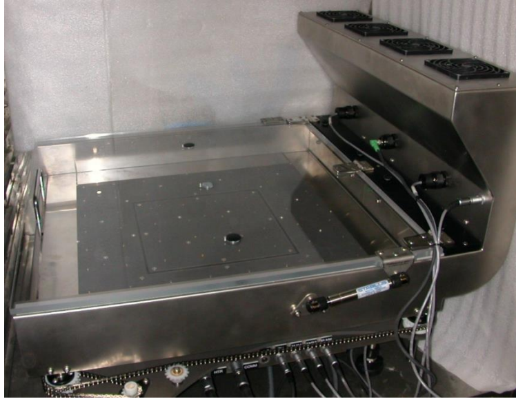
Figure 2.11 The sweating guarded hotplate system
