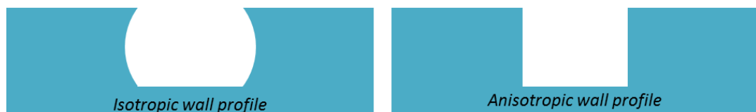
Figure 2.19 - Wall profiles caused by different etching techniques. Wet etching commonly produces an isotropic wall profile, whereas a dry etch will provide a straight anisotropic profile.
