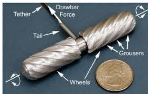
Figure 2.6 - The mobile Nebraska robotic device, which uses metallic wheels to traverse abdominal organs [37].
