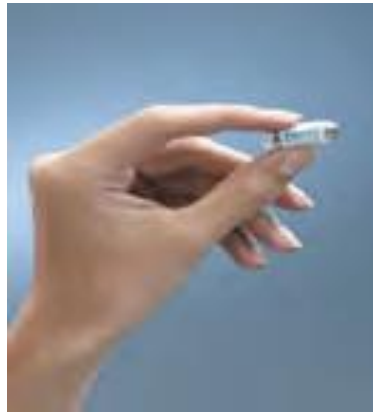
Figure 2.4 - Image of the PillCam device, which has been designed to provide visualisation through the digestive tract [33].
