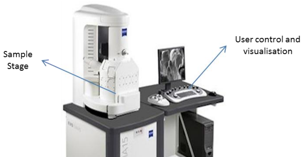
Figure 3.5 - Carl Zeiss EVO SEM with oxford instruments EDX system [117].
