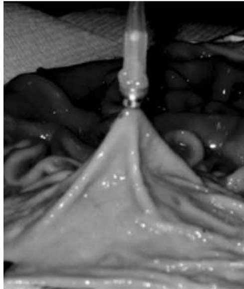
Figure 2.7 - Injection of ferromagnetic fluid into a porcine stomach, an external permanent magnet can be seen to retract the tissue [45].
