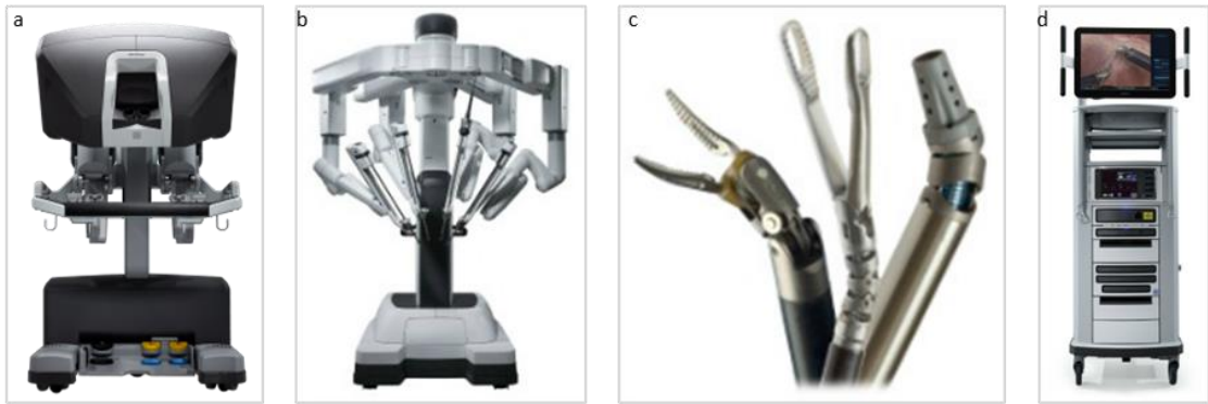
Figure 2.3 - Components of the da-Vinci surgical system, a) the surgeon's console, b) the patient side cart, c) the endowrist instruments and d) the vision system [27]
