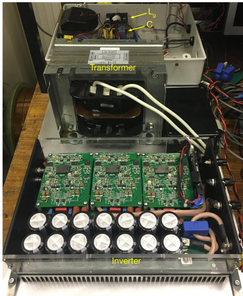
Fig. 3-43 Low frequency transformer based charger hardware setup
