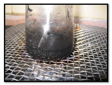
a flame in order to boil the mixture. The liquid was then poured through a filter paper into another beaker. The clear filtrate is evaporated to obtain ingredient 1: saltpetre.
