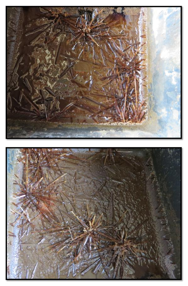
Figure 8: crystals in trough before (above) after (below) draining
