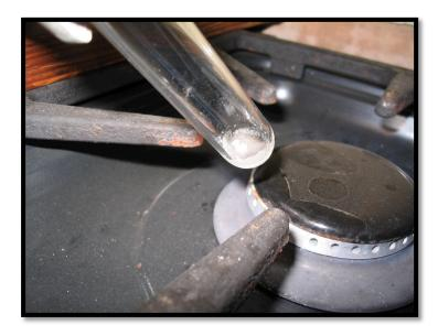
test tube. This causes a bright, hissing reaction. Boyle interpreted this as the 'volatile' acidic component of the nitre being driven off, leaving the 'fixed' alkaline component behind. The addition of coals, we know now, drives away the oxygen from the nitre.
