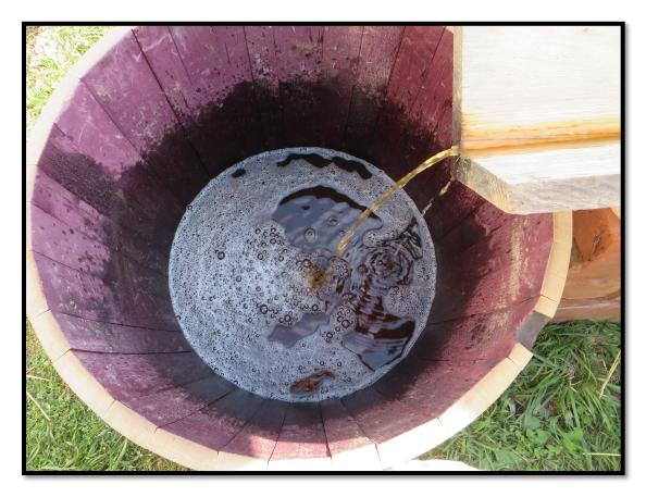
Figure 6: lixivium of four settling tubs draining via the trough
