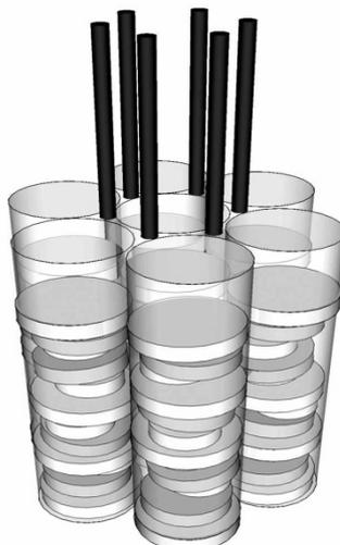
**Figure 6.53** A disordered hexagonal columnar phase made by molecules differing diameters, which are laterally and vertically disorganised along the column axes. The defects between the columns (thick lines) will possess long range periodic ordering.
