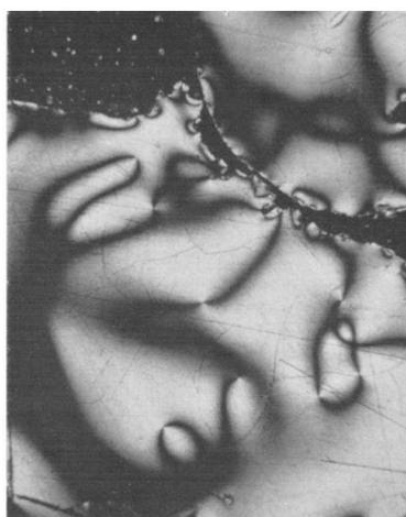
**Figure 1.19** Polarized light micrograph (crossed polarizers) (150 X) of extracted pitch carbonized to 450 °C at approximately 0.4 °C /min.[49]
