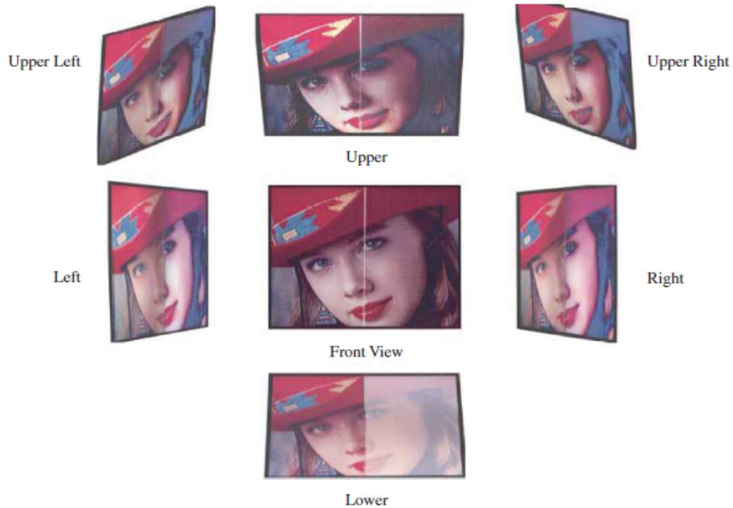
**Figure 1.17** The effect by different angle of view for a Fuji WV optical compensating film on a liquid crystal display.[45]
